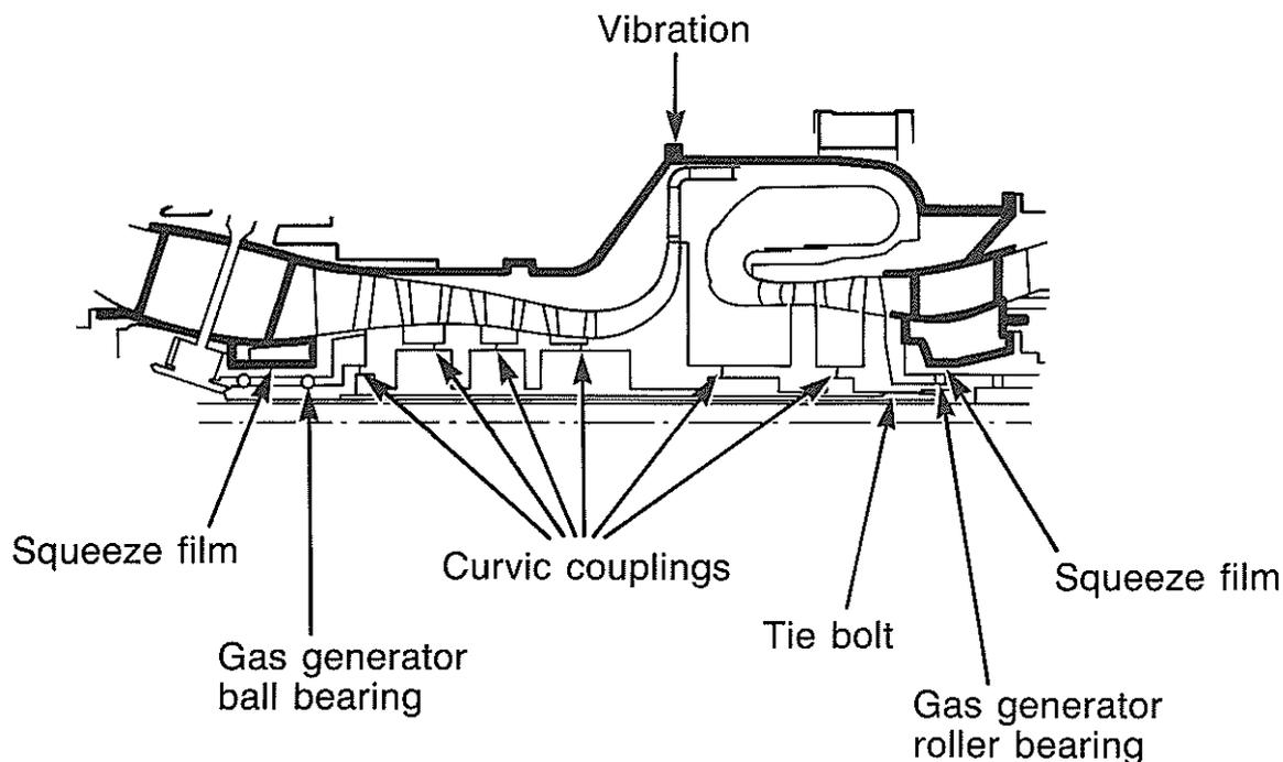
Fig.9 Gas generator shaft arrangement
