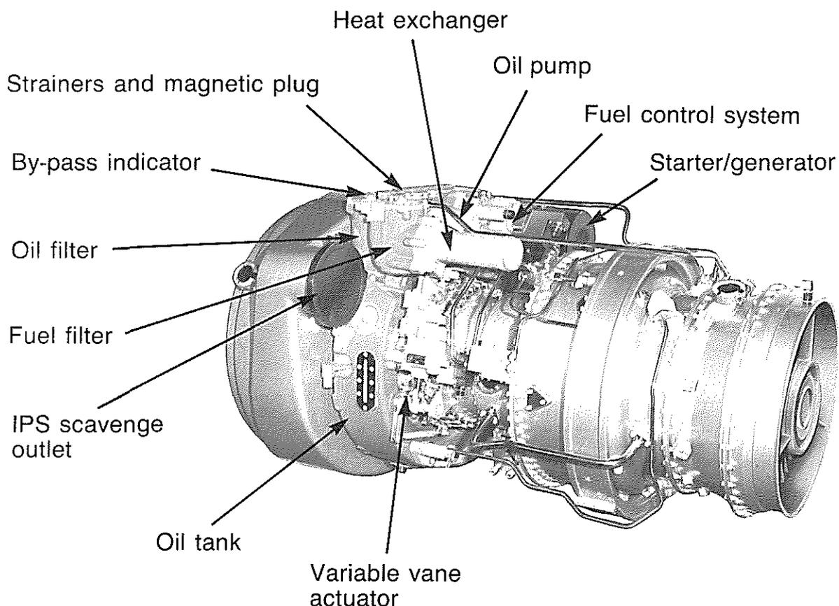
Fig.8 External view of engine
