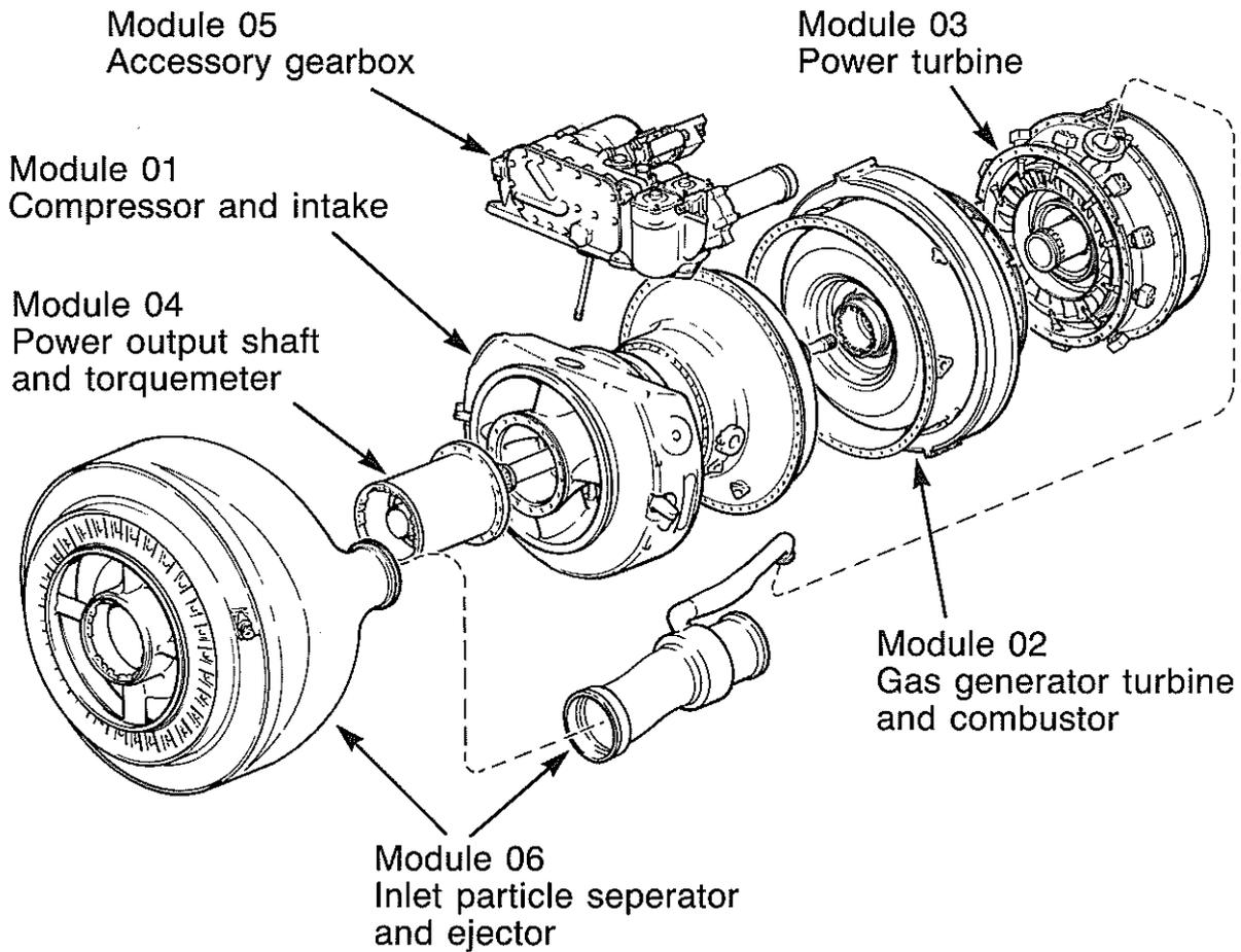
Fig.7 Engine modules
