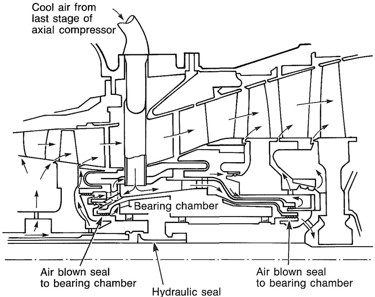
Fig.10 Turbine bearing chamber
