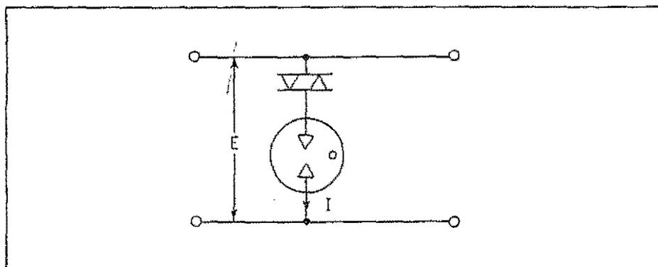
FIG. B - Hybrid Protective Device Made of Varistor and Spark Gap Combination
