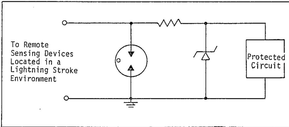
FIG. C. - Spark Gap-Zener Diode Hybrid
