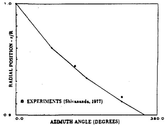
Figure 5. Comparison of tip vortex location with experiments of Ref. 26
