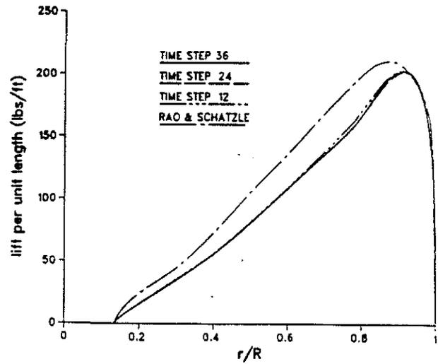
Figure 3. Development of blade loading
