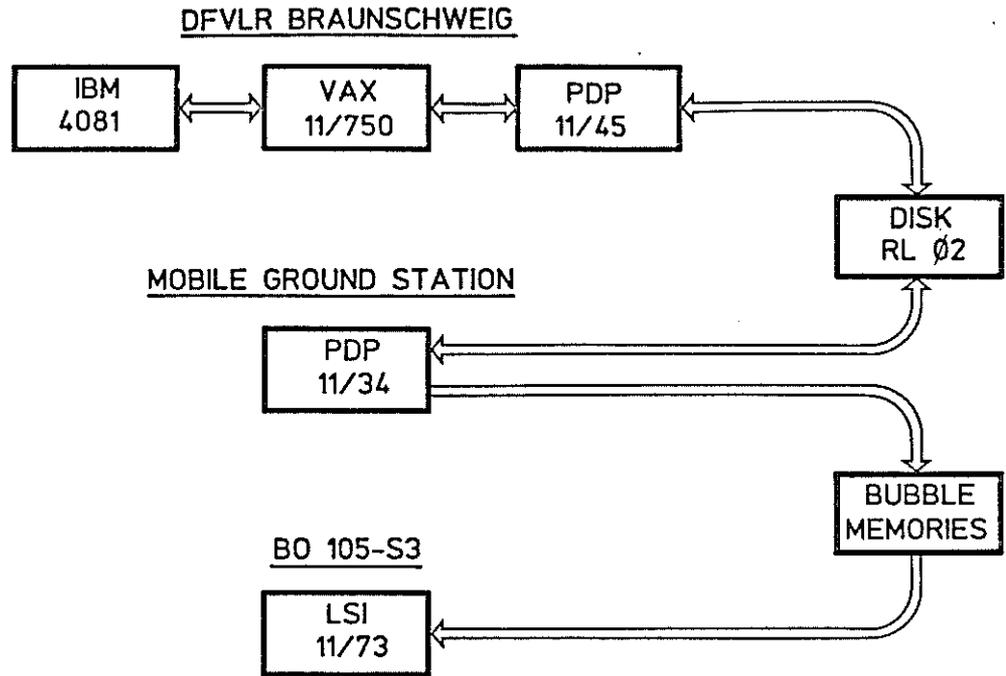
Figure 4: Simulation Software Data Flow
