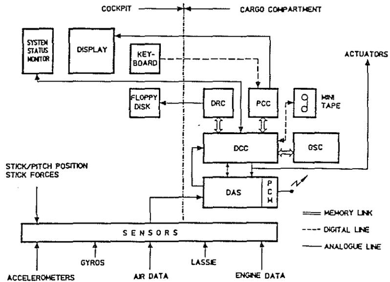
Figure 3: Realized MFCS System Structure
