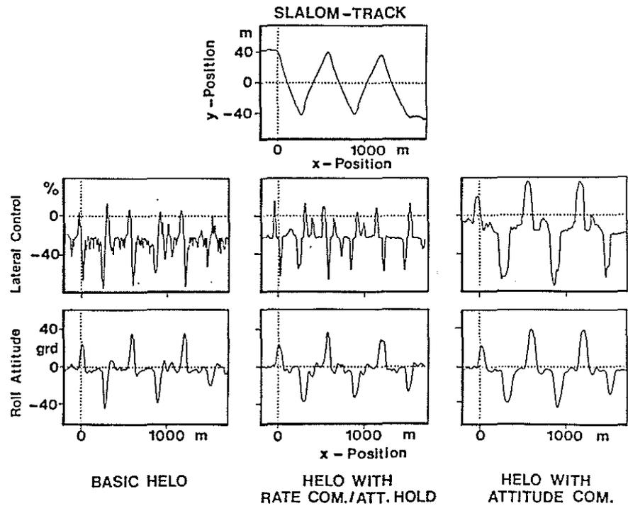
Figure 9: Time Response of Different Models in the Slalom Task
