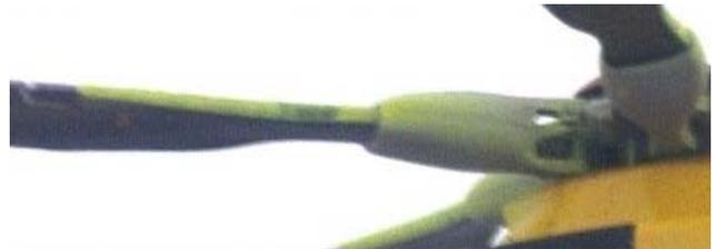
Figure 13 - Unheated sections of main rotor blade
