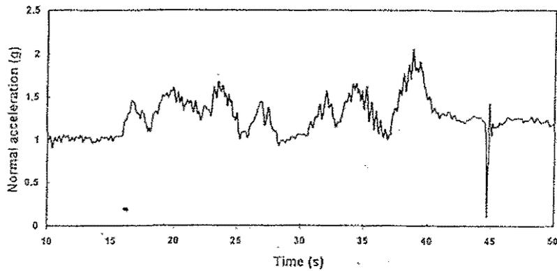
Figure 12 - Slalom MTE Associated Normal Acceleration
