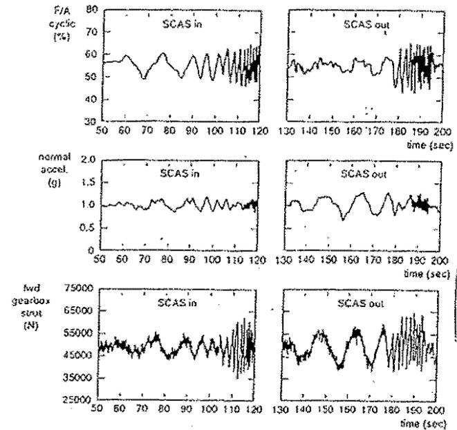
Figure 5 - Frequency Sweep on DRA Research Puma - 60kn SCAS on and off.
