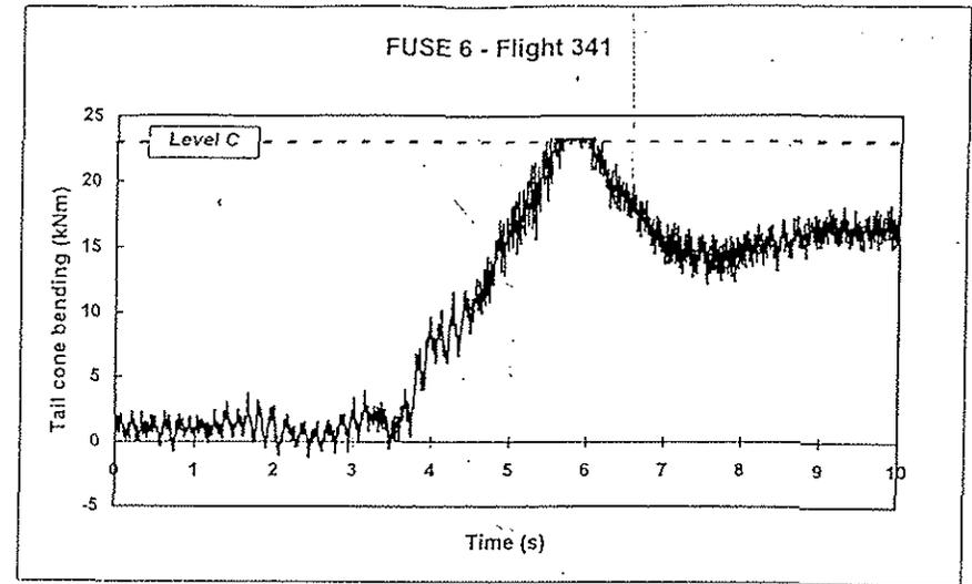
Figure 9 - Deceleration to Dash MTE Tail Cone Bending Level 'C' Exceedence
