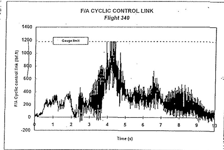
Figure 10 - Transient Turn F/A Cyclic Control Link Level 'C' Exceedence
