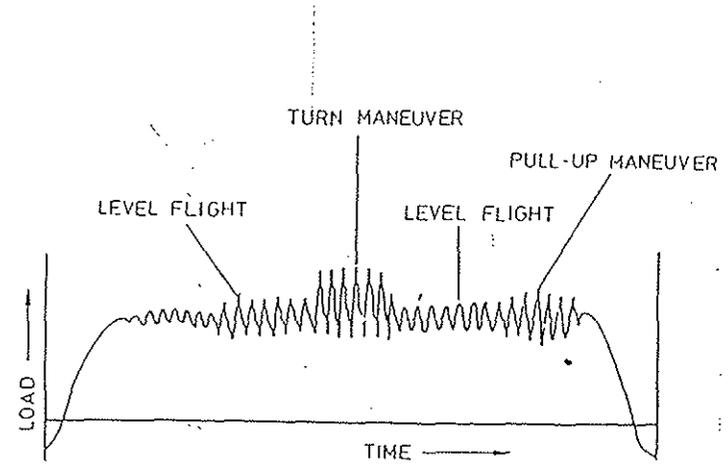
Figure 2 - Manoeuvre and Mean Cyclic Loads
