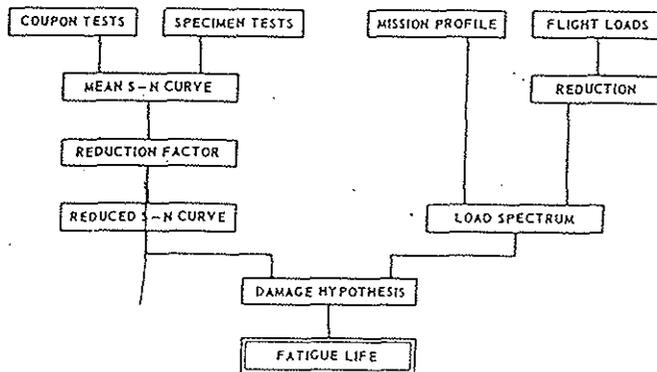
Figure 1 - Fatigue Substantiation Methodology
