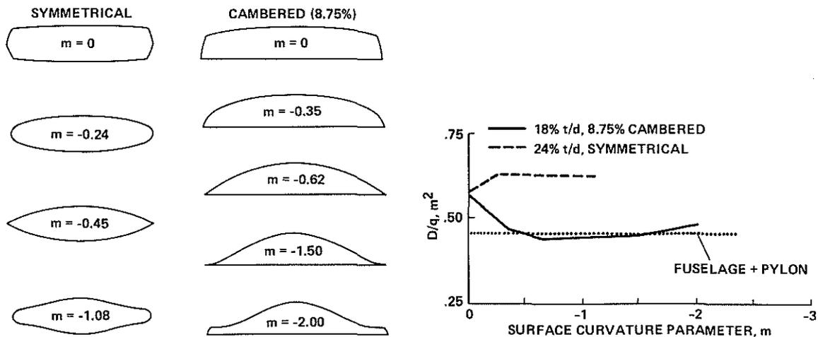
Figure 11 - Effect of hub-fairing cross-sectional shape on drag at  $\alpha = -2^\circ$ .
