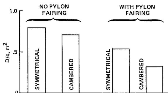
Figure 7 - Comparison of drag levels with symmetrical and cambered hub fairing.
