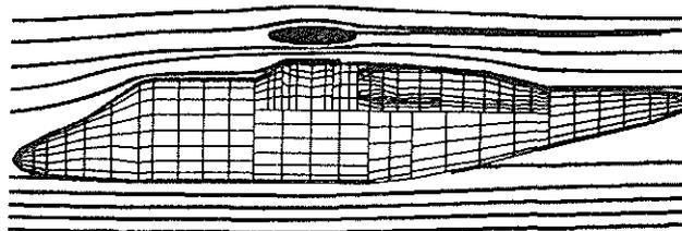
Figure 5 - Flow field about fuselage with symmetrical hub fairing.
