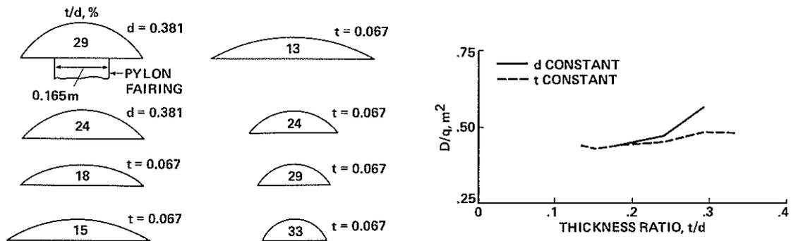
Figure 10 - Effect of hub-fairing thickness-to-diameter ratio on drag at  $\alpha = -2^\circ$ .
