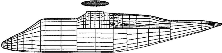
Figure 1 - Symmetrical hub fairing atop helicopter fuselage.
