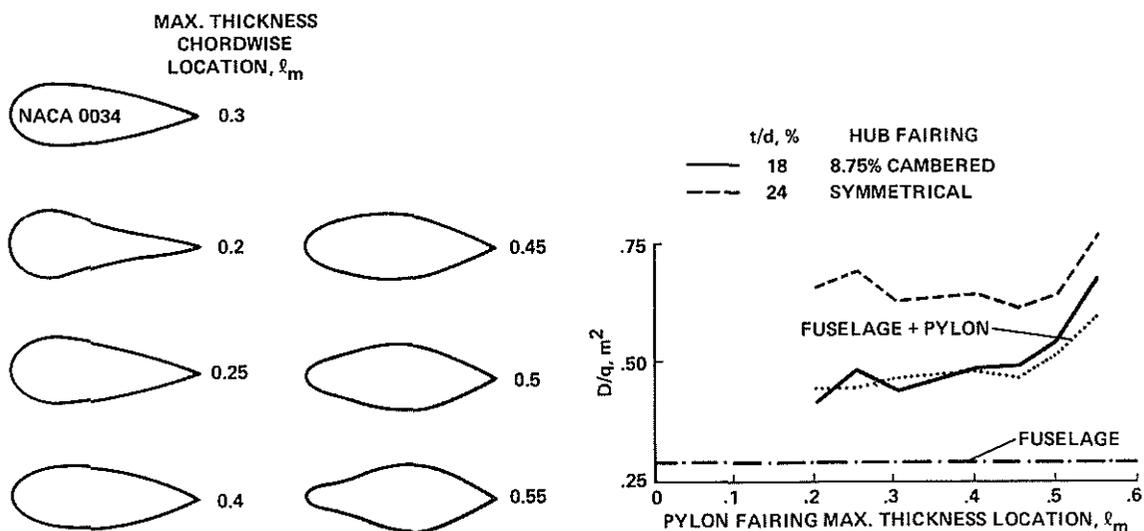
Figure 12b - Effect of pylon configuration on drag at  $\alpha = -2^\circ$ .
