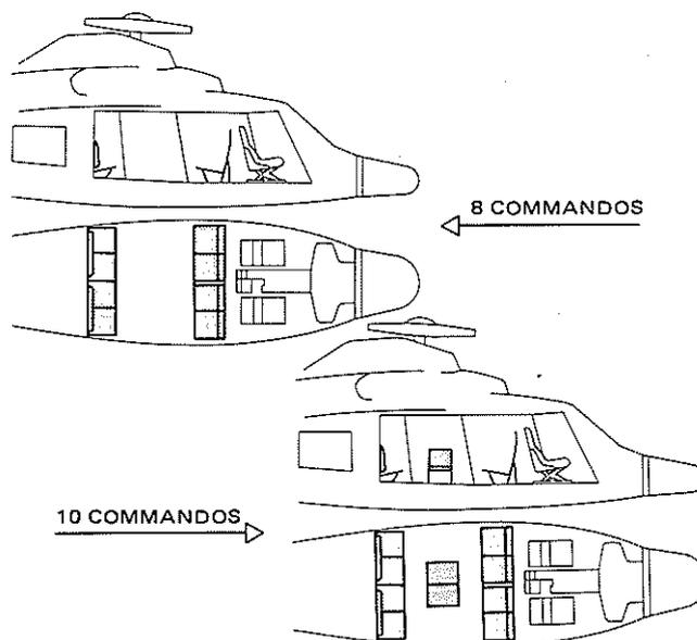
Fig. 3 : COMMANDO TRANSPORT LAYOUT
