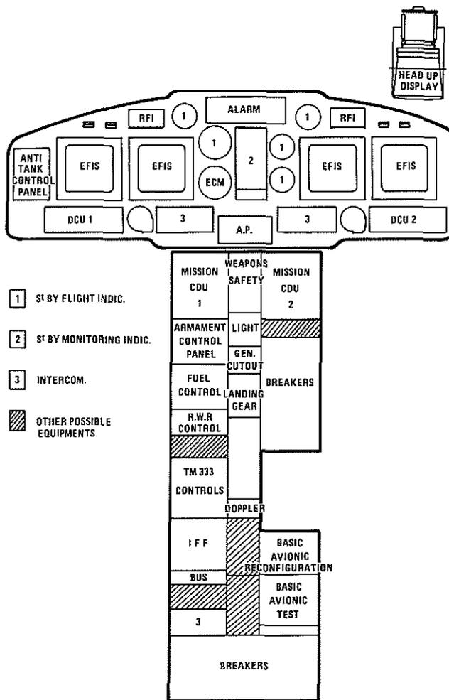
Fig. 16b : EXAMPLE OF INSTRUMENT PANEL INCORPORATING 4 MULTI-FUNCTION DISPLAY UNITS
