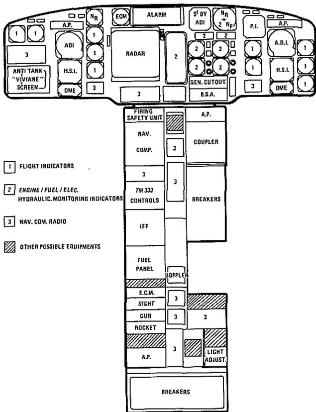
Fig. 16 : INSTRUMENT PANEL AND CONSOLE
