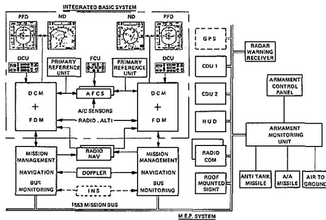
Fig. 16a : EXAMPLE OF DIGITAL SYSTEM FOR AN ANTI-TANK / ANTI-HELICOPTER VERSION
