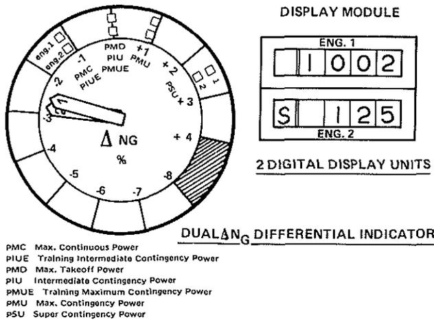
Fig. 15c : ENGINE MONITORING EQUIPMENT ON INSTRUMENT PANEL
