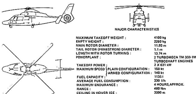
Fig. 2 : SA 365 M PANTHER CHARACTERISTICS
