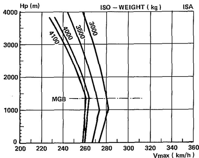
Fig. 22 : MAXIMUM CONTINUOUS SPEED ( ISA ) IN ARMED CONFIGURATION ( TWO 20 mm CANNON PODS )
