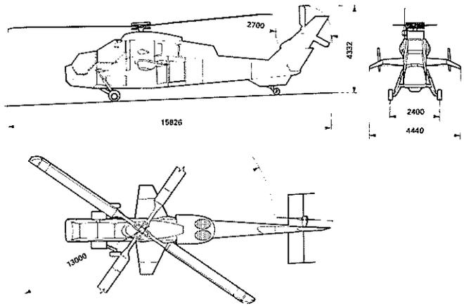
Fig. 8: THREE-VIEW DRAWING (BASIC HELICOPTER)
