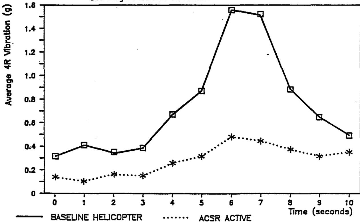
**FIGURE 11. Westland 30 Flight Test, ACSR Performance for Transition to Hover Manoeuvre**
