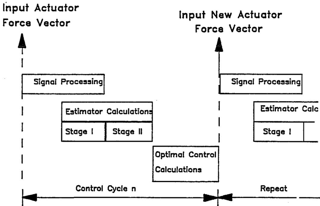
**FIGURE 2. Control System Timing Diagram**
