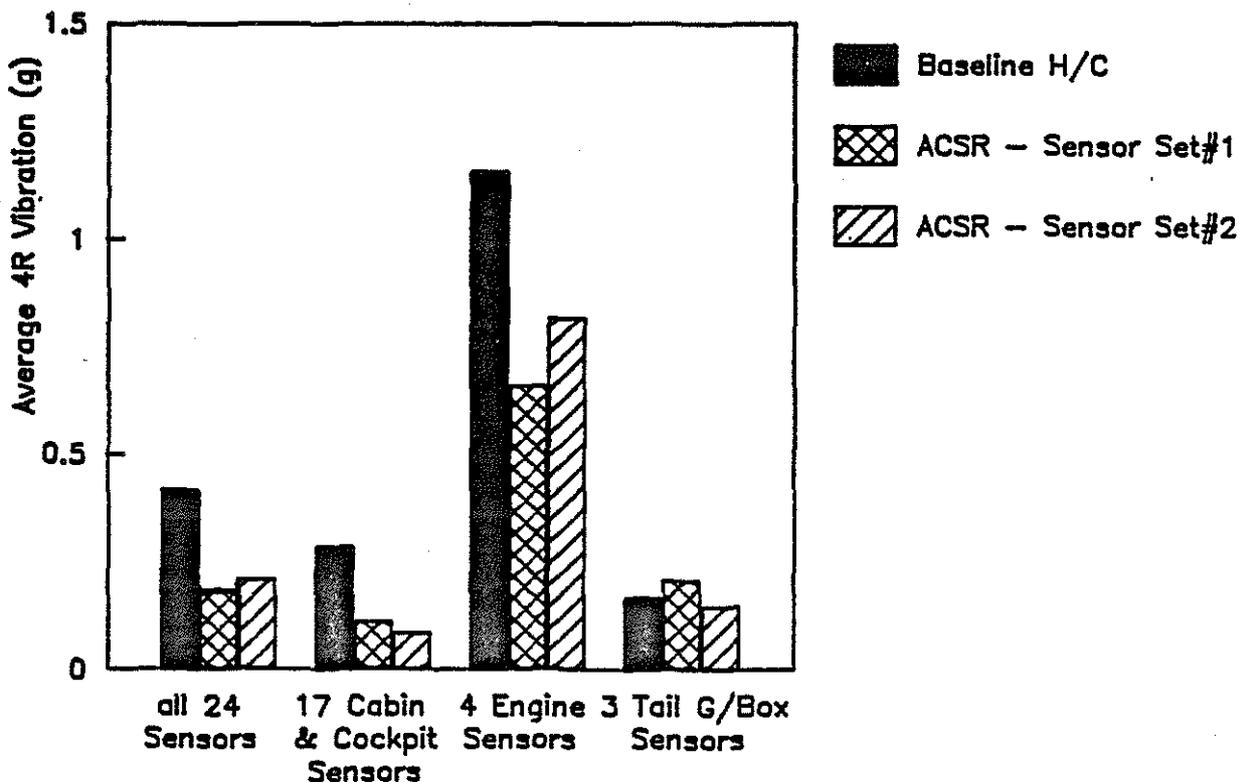
**FIGURE 7. Westland 30 Flight Test, Effect of ACSR Sensor Selection @ 80 knots**
