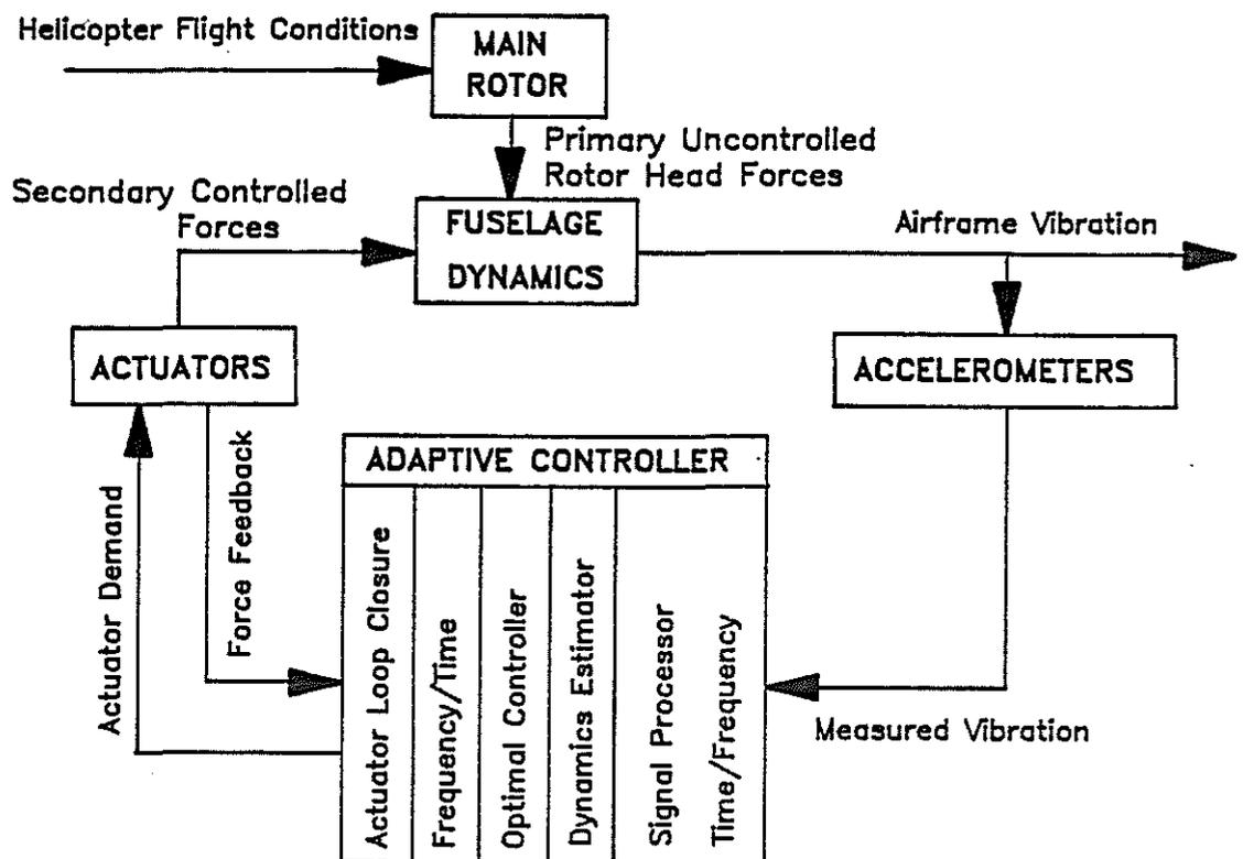
**FIGURE 1. ACSR Helicopter System Schematic**
