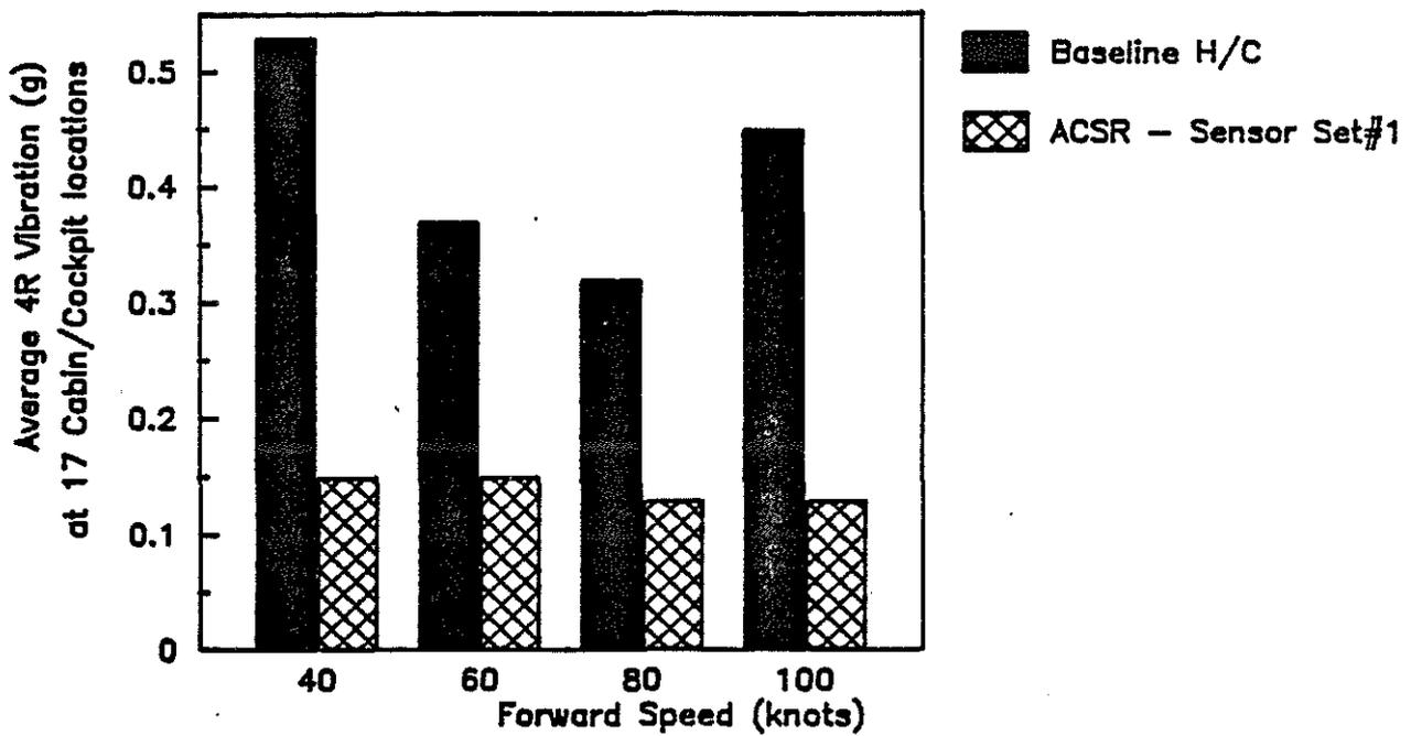
**FIGURE 10. Westland 30 Flight Test, ACSR Performance for Modified Aircraft Weight and Distribution**
