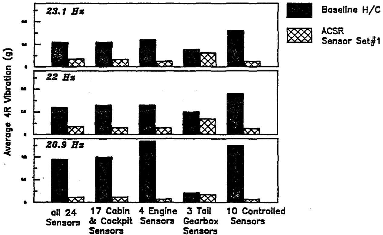
**FIGURE 6. Westland 30 ACSR Ground Vibration Test, Performance for 900 N-m Roll Moment**
