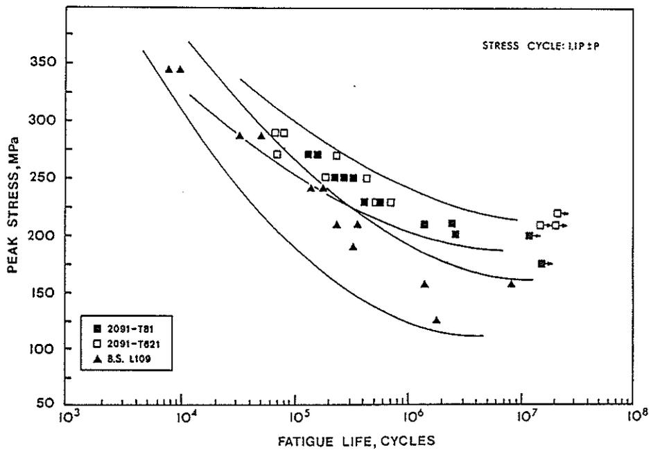
Figure 4. Comparison of fatigue behaviour of BS L109 sheet with that of (a) stretched and (b) re-solution treated recrystallised AA2091 sheet in the LT direction and aged 12h at 135°C.
