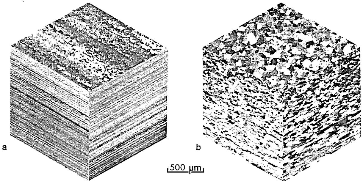
Figure 2. Aluminium-lithium alloy grain structures (a) Unrecrystallised (b) Recrystallised.
