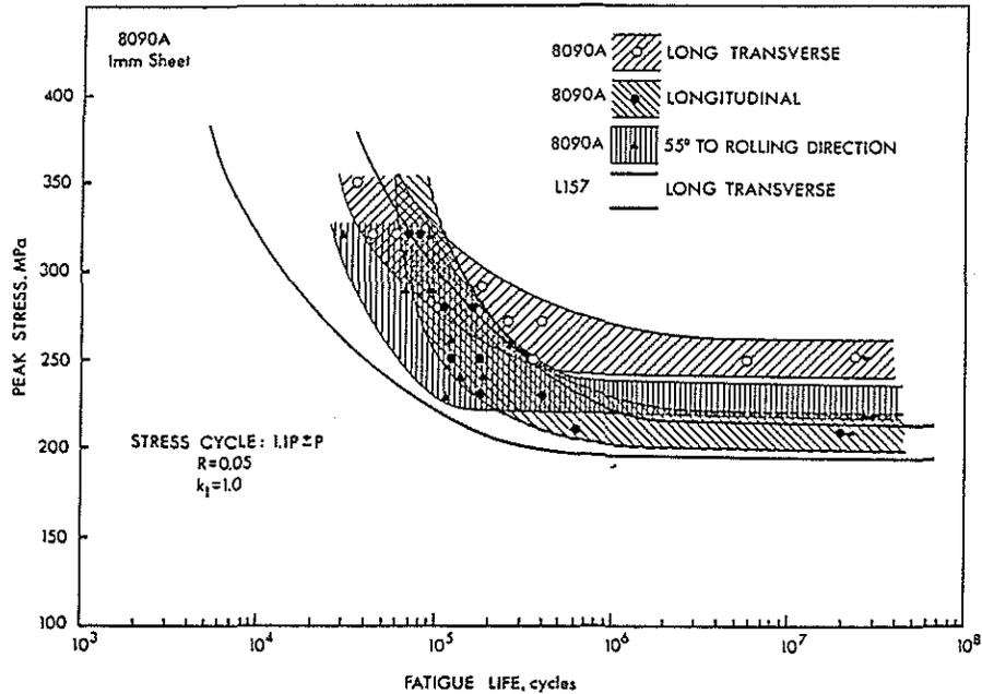
Figure 7. S-N curves of 8090A stretched sheet aged 30h at 175°C.
