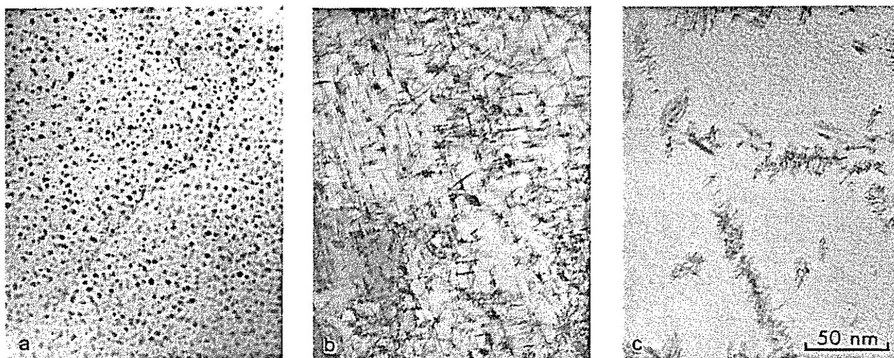
Figure 1. Typical Al-Li-Cu-Mg-Zr alloy TEM micrographs (a)  $\delta'$ - $Al_2Li$  precipitates (b)  $S'$ - $Al_2CuMg$  precipitates in metal with cold working operation (c)  $S'$ - $Al_2CuMg$  precipitates in metal without cold working operation.
