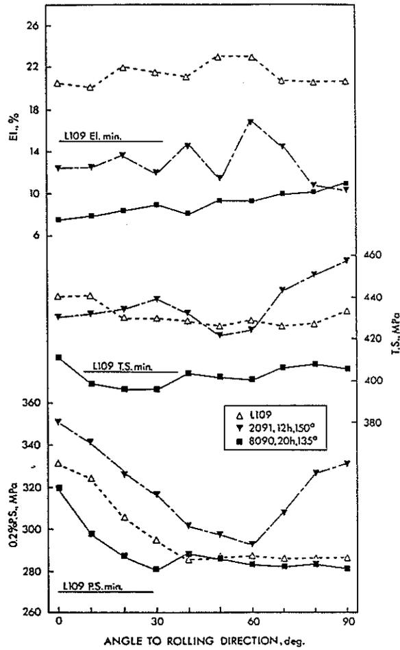
Figure 3. Anisotropy in 2091 and 8090C sheet aged to the 'damage tolerant' condition, with L109 data for comparison.
