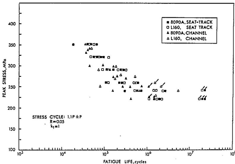
Figure 13. S-N curves for 8090 and BS L160 C-channel and seat track extrusions.
