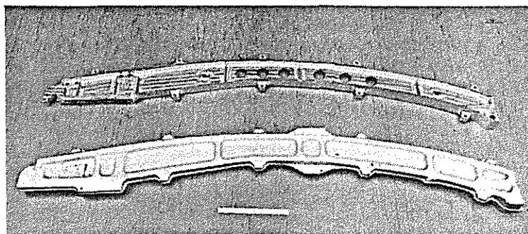
Figure 8. EH101 Cabin Frame forgings before and after machining.
