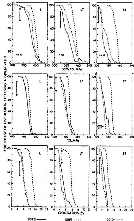
Figure 10. Proportion of forging static properties exceeding a given value.
