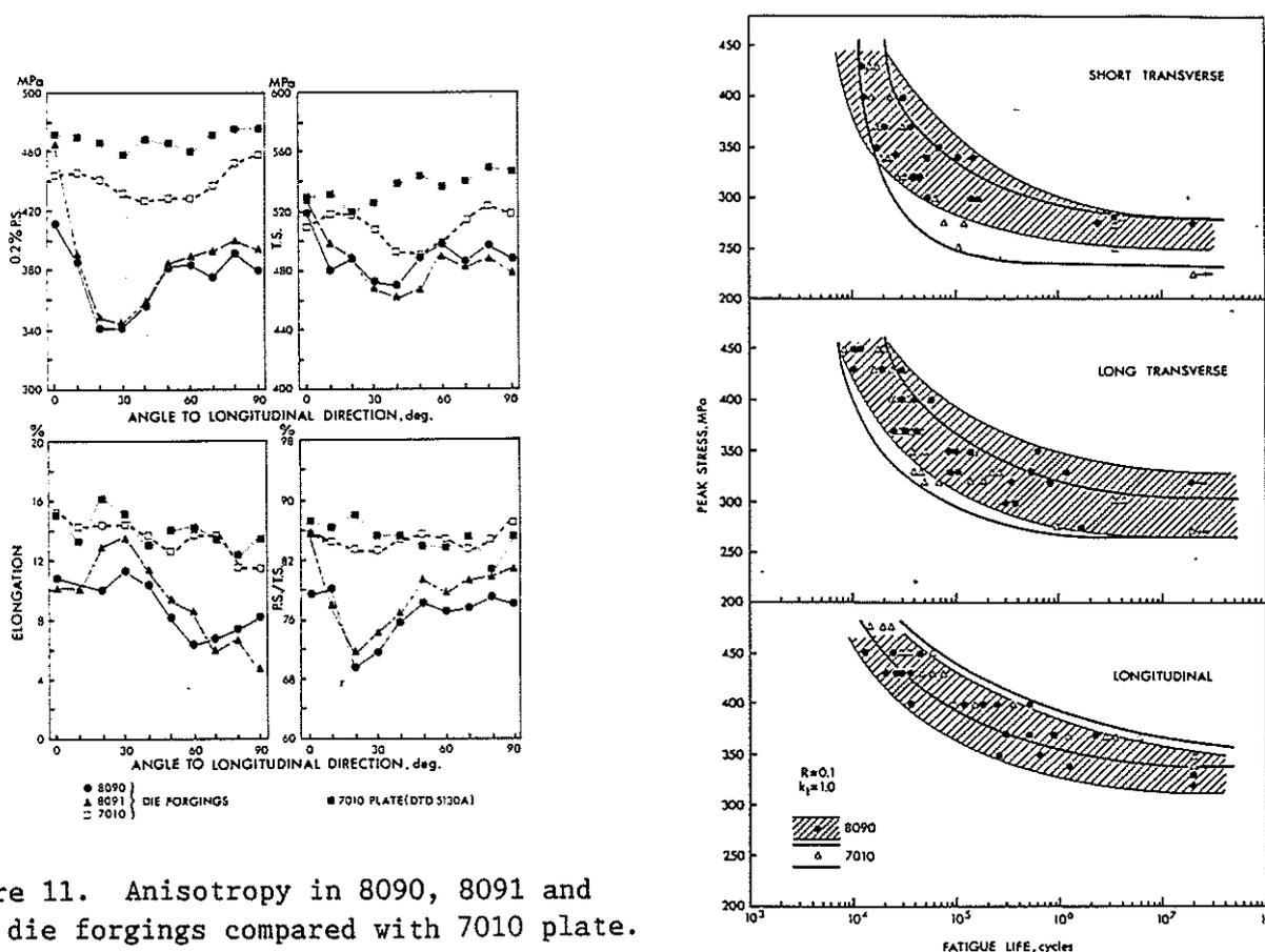
Figure 11. Anisotropy in 8090, 8091 and 7010 die forgings compared with 7010 plate.
