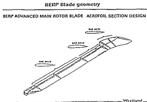
The advanced tip uses the thin RAE 9634 section. The leading edge notch formed at the transition of the aerofoils at the tip acts as a low drag aerodynamic fence. This prevents flow separations initiated by stall at the inboard sections propagating into the tip region. The sharp sweepback at the outboard edge of the tip promotes vortex flow at high angles of attack and prevents the tip from stalling conventionally. (See Figure below).
