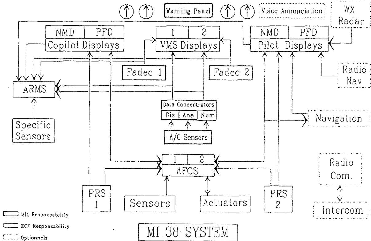
MI38's system architecture is based on ARINC 429 data links with the exception of specific equipment e.g. weather radar for which special standards are defined.
