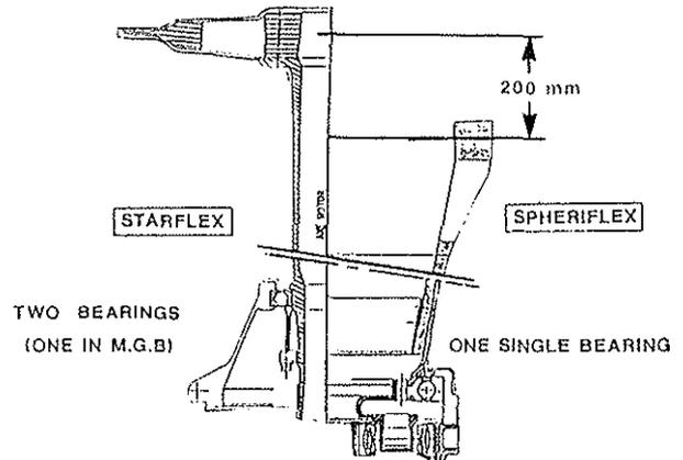
Fig. 5 : MOUNTING OF THE MAST ON THE MGB
