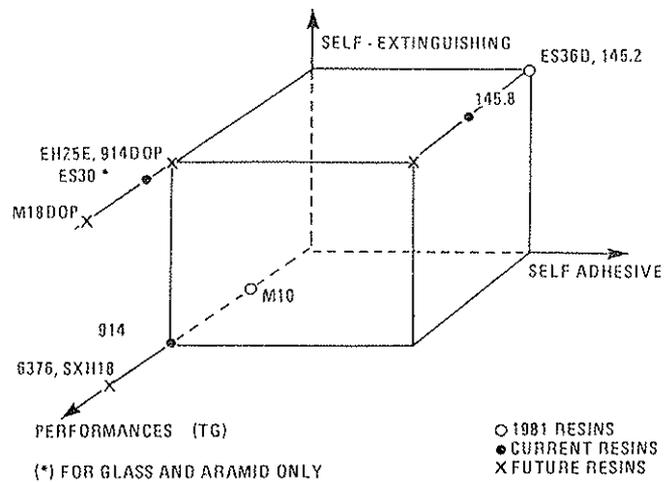
Figure 11- Resins for Use in Primary Structures
