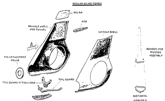
Figure 14- 350Z Composite Fenestron and Fin
