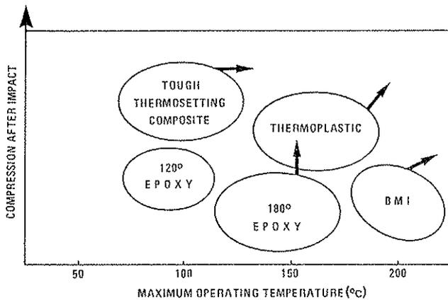
Figure 10- Thermosetting and Thermoplastic Composite Performances
