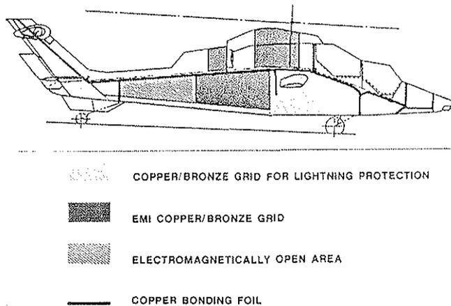
Figure 4 - Lightning and Electromagnetic Protection
