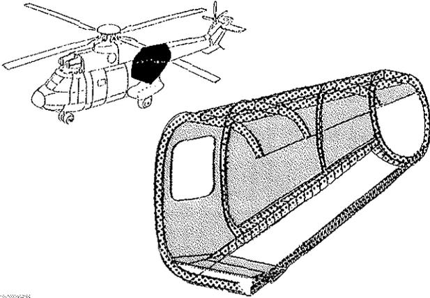
Figure 25- AS332 MKII Intermediate Composite Structure
