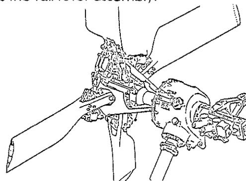
Fig. 15: Tail Rotor Assembly
