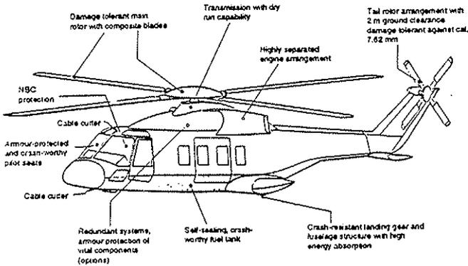
Fig.10: Technologies applied to NH90
