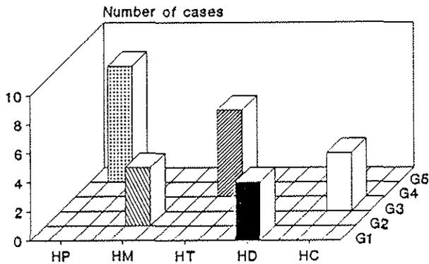
FIG.9 FAULT CLASSIFICATION BASED ON THREE NORMALIZED VIBRATION COMPONENTS
