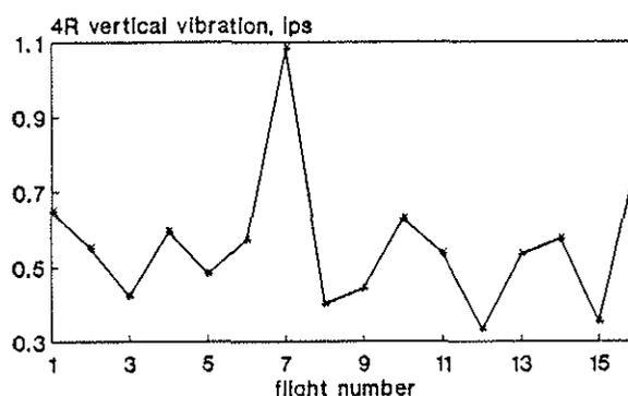
FIG.1 MEASURED 4R AIRFRAME VIBRATION (SPS SENSOR LOCATION), AS332L IN THE CRUISE
