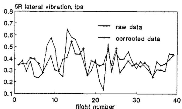
FIG.4 MEASURED AND CORRECTED 5R AIRFRAME VIBRATION (SPS SENSOR LOCATION), S61 IN THE CRUISE
