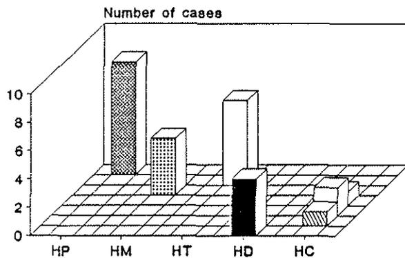
FIG.10 FAULT CLASSIFICATION BASED ON 15 NORMALIZED VIBRATION COMPONENTS
