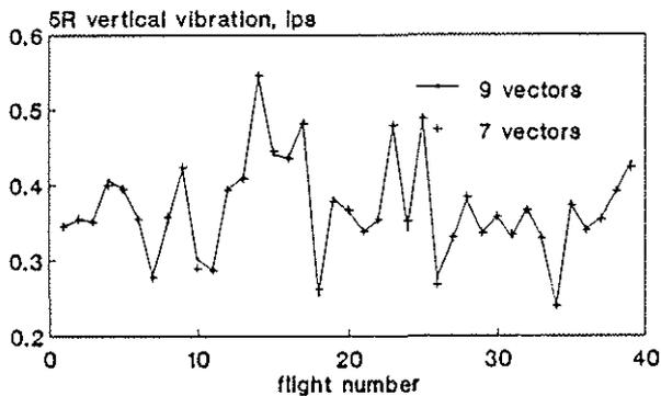
FIG.5 CORRECTED VIBRATION USING 7 AND 9 EIGEN VECTORS IN THE PREDICTION MODEL, S61 IN THE CRUISE
