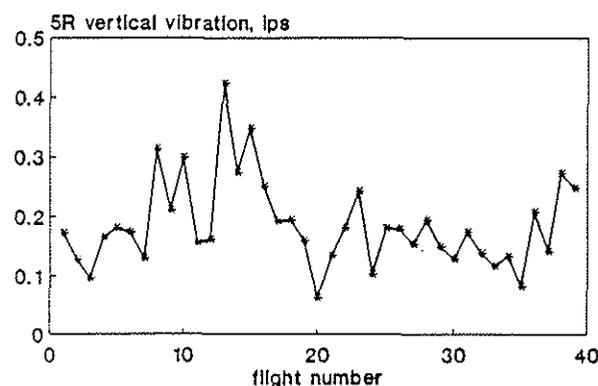
FIG.2 MEASURED 5R AIRFRAME VIBRATION (SPP SENSOR LOCATION), S61 IN THE CRUISE
