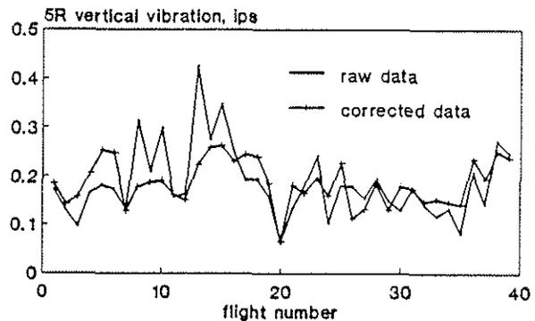
FIG.3 MEASURED AND CORRECTED 5R AIRFRAME VIBRATION (SPP SENSOR LOCATION), S61 IN THE CRUISE
