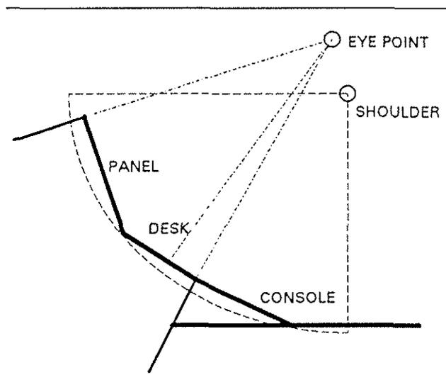
Fig.2 XZ plane cockpit cross section, internal vision and reach layout.
