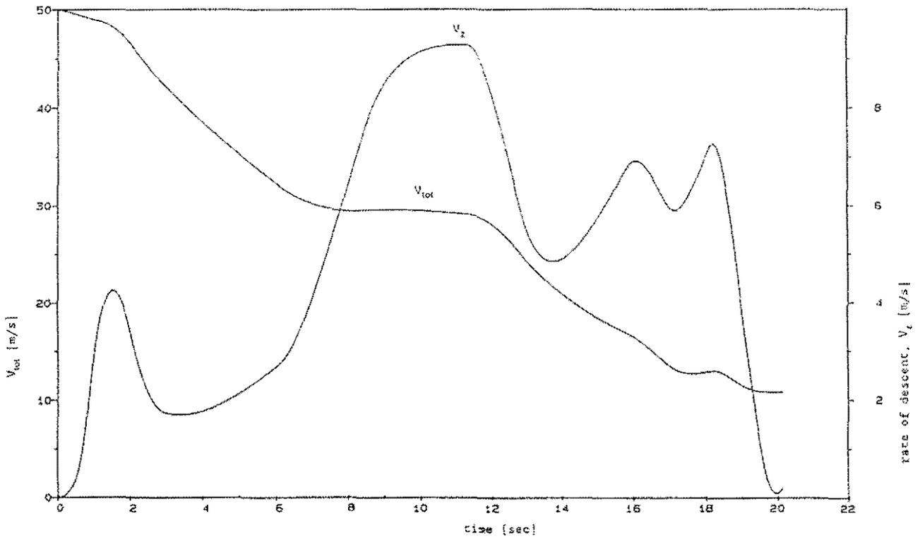
Figure 7: Velocity and rate of descent as function of time.
