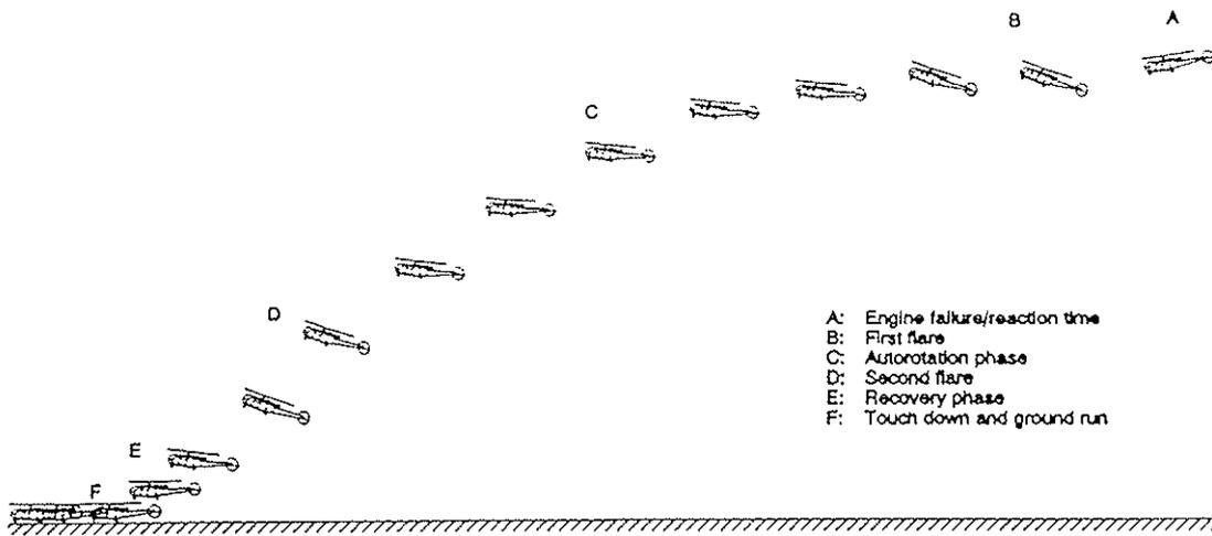
Figure 2: General lay out of the standard autorotative flight.
