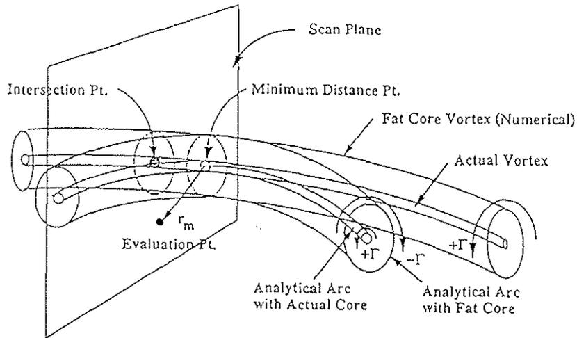
Figure 6. Schematic showing superposition of the low-resolution numerical solution and high resolution analytical solution for the nearfield velocity correction.
