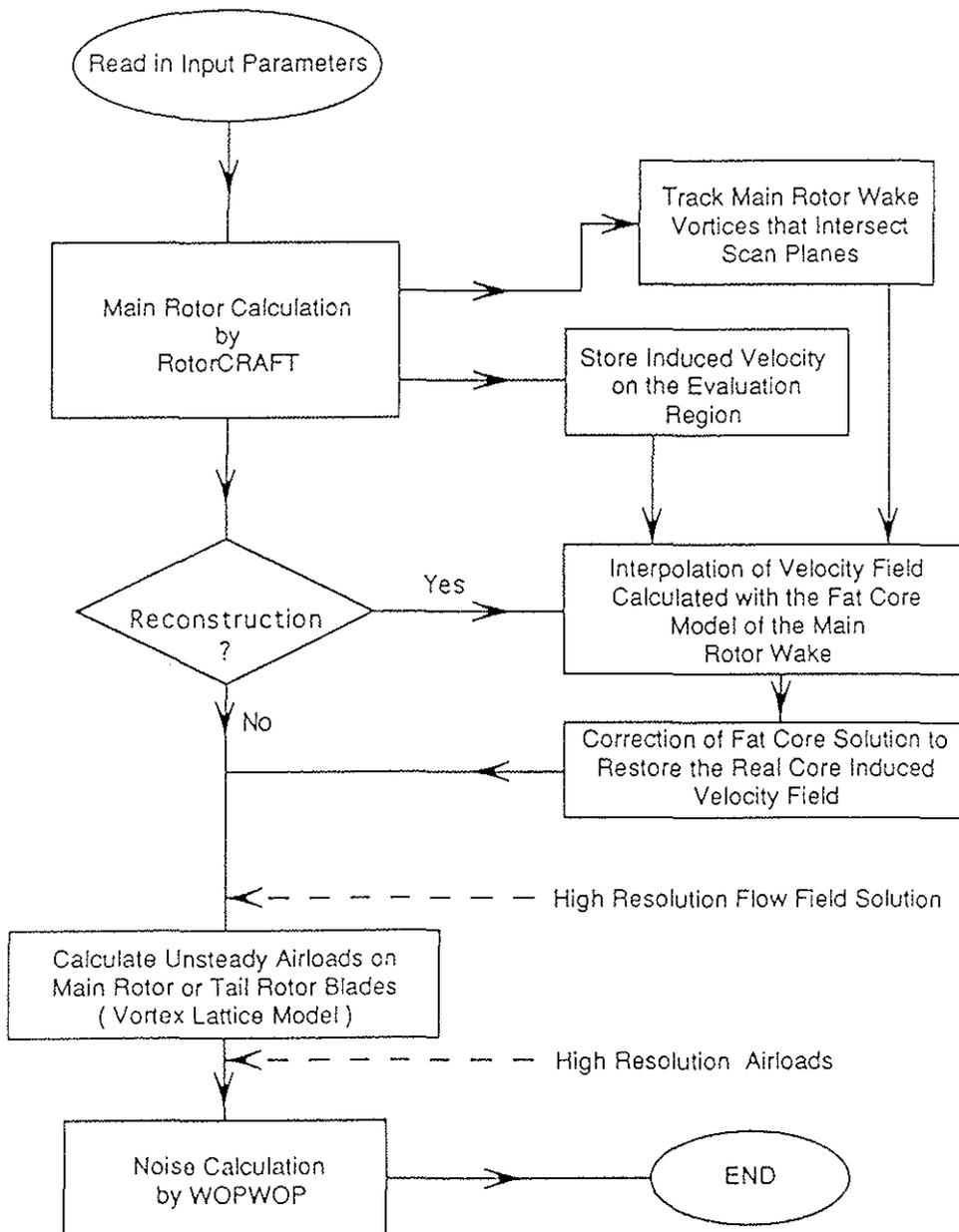
Figure 5. Simplified flow chart of program modules used for flow field and airload reconstruction.
