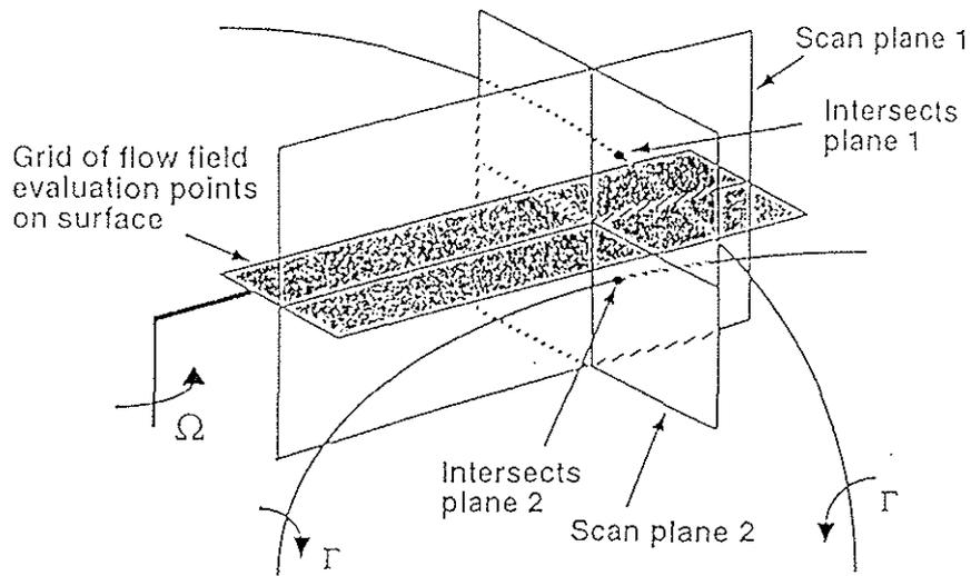
Figure 4. Typical orientation of scan planes attached to a moving blade to capture parallel and perpendicular vortex interaction events.
