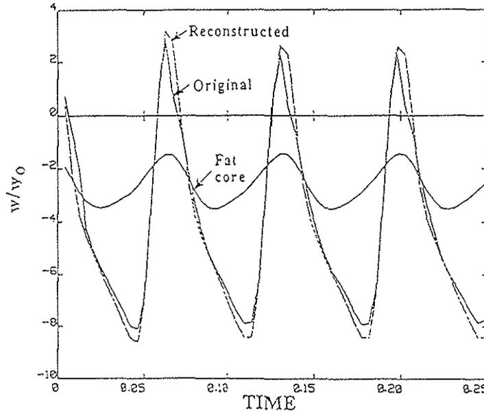
Figure 7. Comparison of actual, reconstructed and fat core downwash at a fixed point corresponding to the advancing blade tip for an H-34 at  $X/R = 0.0$ ,  $Y/R = 1.0$ . 4:1 time interpolation used.
