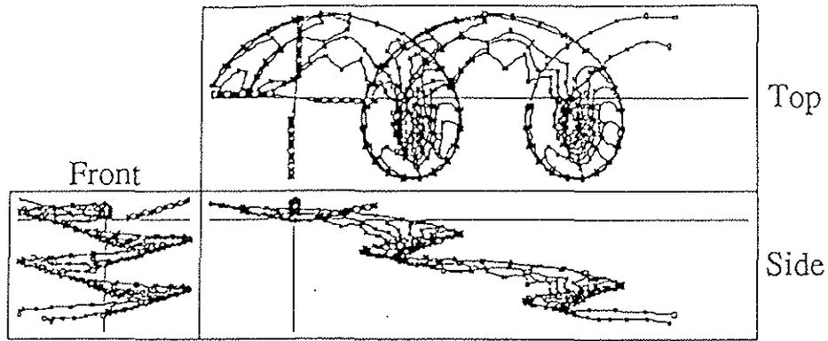
Figure 1. Wake geometry for one blade of a four-bladed rotor at advance ratio 0.3 using the Constant Vorticity Contour (CVC) wake model. (Only two turns of the full-span CVC wake are shown; vertical scale expanded by a factor of 5.0.)
