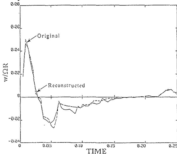
Figure 8. Original and reconstructed downwash at  $r/R = 0.9$  on one blade of an H-34 rotor. 4:1 time interpolation used.
