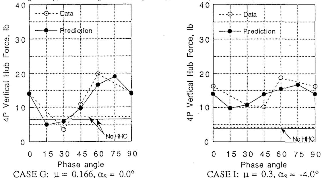
Figure 3. Comparison of predicted and experimental 4P vertical hub force amplitude for 4P HHC input of amplitude  $\theta_c = -0.6^\circ$  as a function of phase angle.
