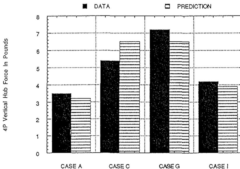
Figure 2. Comparison of predicted and experimental 4P vertical (hub) force amplitude using the RotorCRAFT code. CASE A ( $\mu=0.166$ ,  $\alpha_S=6.0^\circ$ ), CASE C ( $\mu=0.300$ ,  $\alpha_S=2.0^\circ$ ), CASE G ( $\mu=0.166$ ,  $\alpha_S=0.0^\circ$ ), CASE I ( $\mu=0.300$ ,  $\alpha_S=-4.0^\circ$ ).
