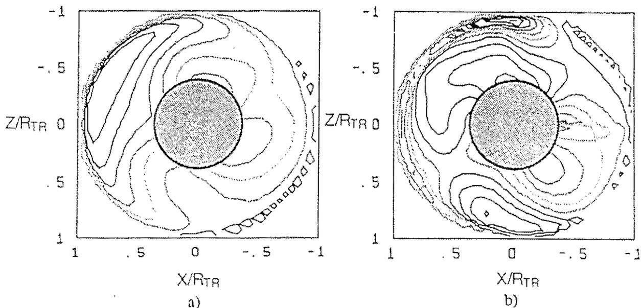
Figure 10. Prediction of surface pressure coefficient at 2% chord on the Puma tail rotor using two different models of tail rotor inflow.
