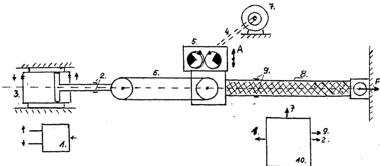
Fig. 2. Test stand for fatigue tests acc. to "gag" method.
