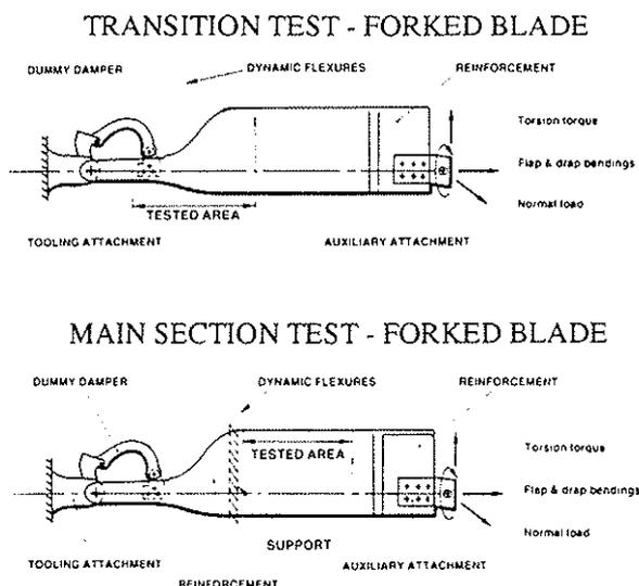
Figure 17. Forked blade tests
