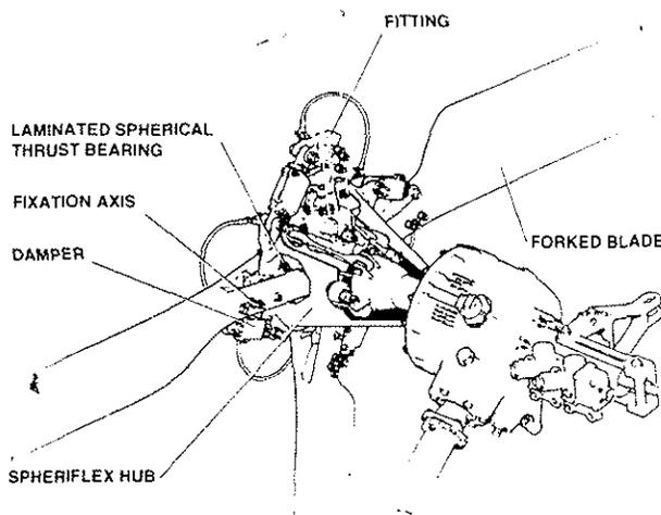
Figure 10. SpheriFlex tail rotor head
