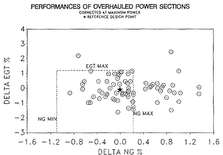
It seems that the behavior of the overhauled engines, having used components assembled together with new ones, very often is different respect to a completely new engine, and the amount of such difference is hard to quantify, due to the deteriorated aerodynamic performances of the compressor and turbine static and rotating blade-rows, caused by the erosion effects suffered during the operative life.
