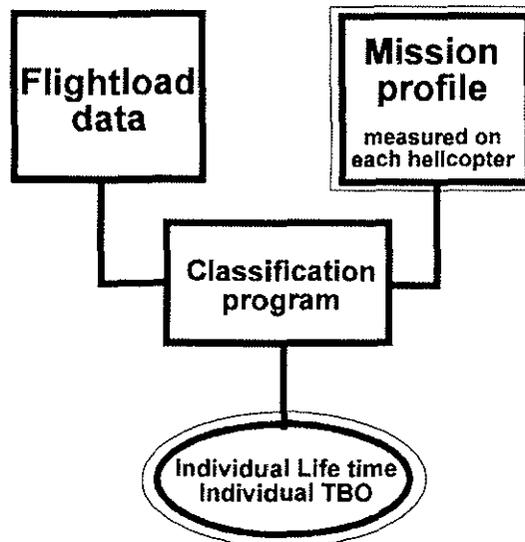
Fig. 4: Life time calculation with flight state recognition
