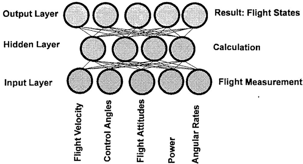
**Fig. 5: The structure of a neural network with neurones and connections between each neurone**
