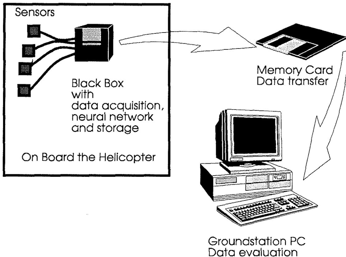
**Fig. 9: Example for a system application including the ground station**
