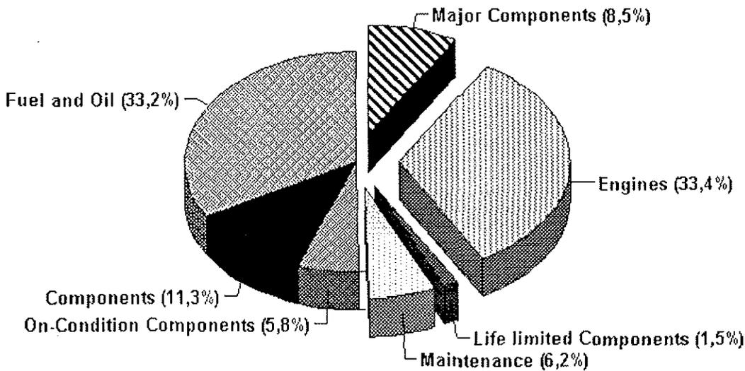
Fig. 2: DOC of a Helicopter and the parts of the DOC which can be influenced by HUMS (BK117 statistical data 1992)
