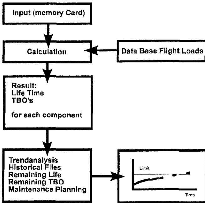
Fig. 10: Functional structure of the ground station software
