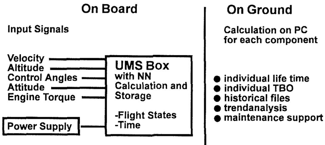
Fig. 7 Principle structure of a usage monitoring system for flight state recognition
