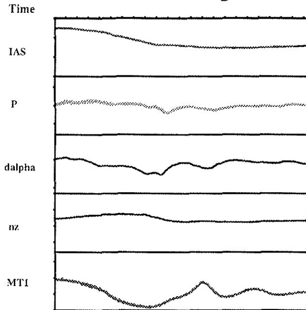
Fig.6: Example of measurement input signals for steady and transient flight states
