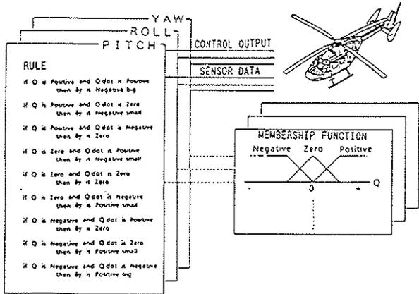
Figure 4 Rate control block
