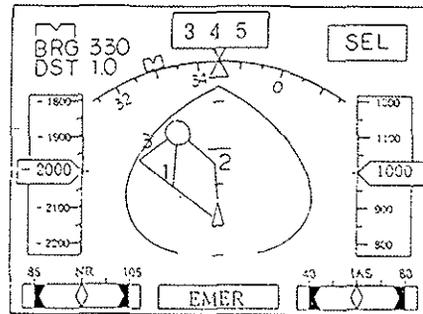
(c) Engine failure 2; recommended flight courses
