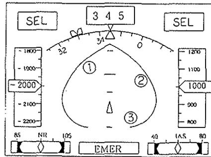
(b) Engine failure 1; reachable range and landing points
