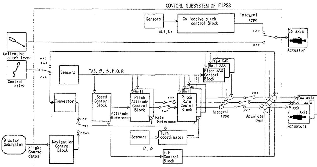
Figure 5. Block diagram of control subsystem
