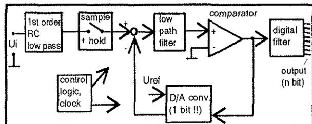
Fig.7: Delta Sigma ADC
