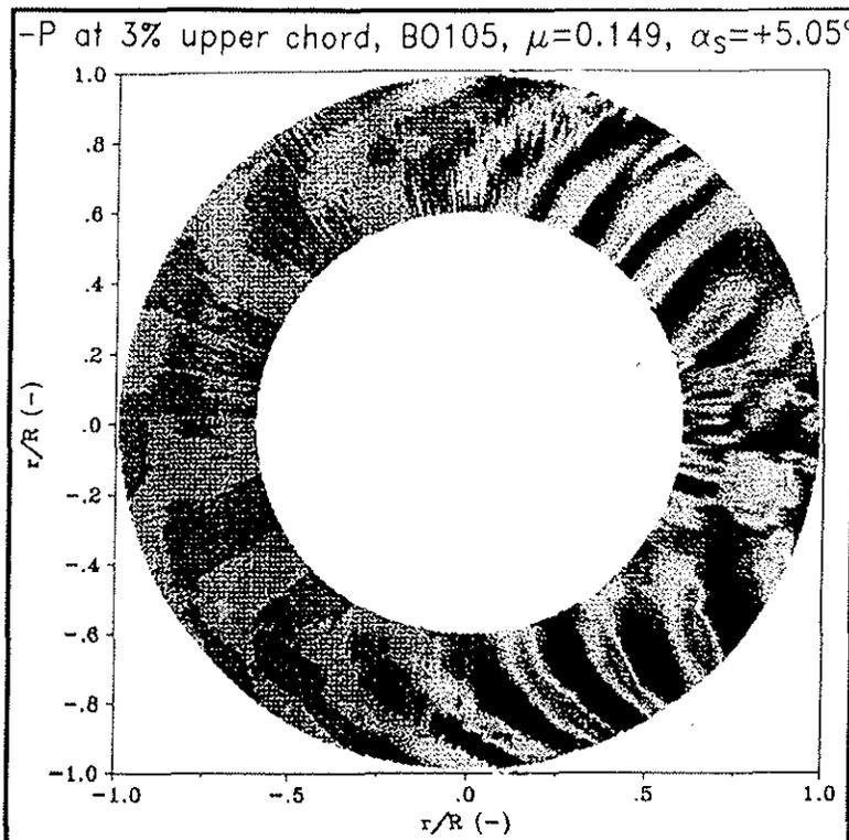
Fig.25: Leading edge pressure distribution with BVI effects
