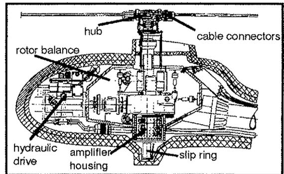
Fig.2: The rotor test rig
