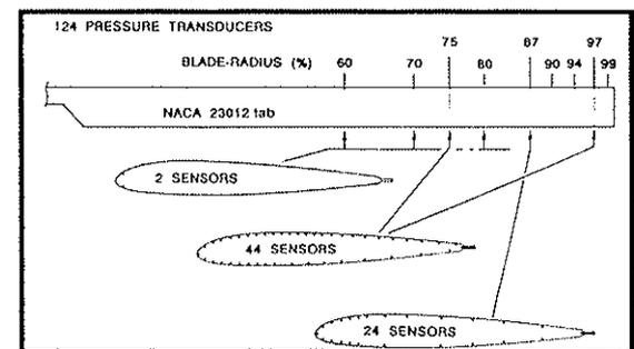
Fig.3: Pressure transducer distribution
