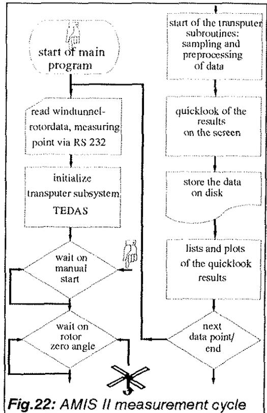
Fig.22: AMIS II measurement cycle
