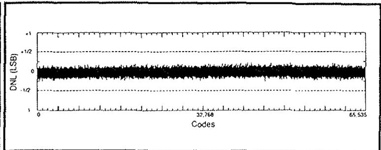
Fig.16: ADC differential nonlinearity
