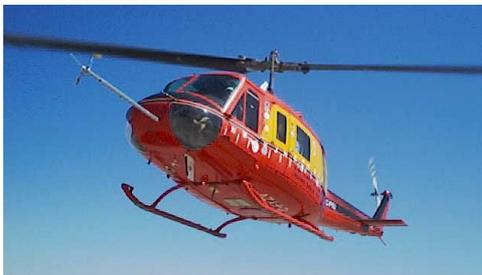
*Fig. 1 Bell 205 Airborne Simulator*
