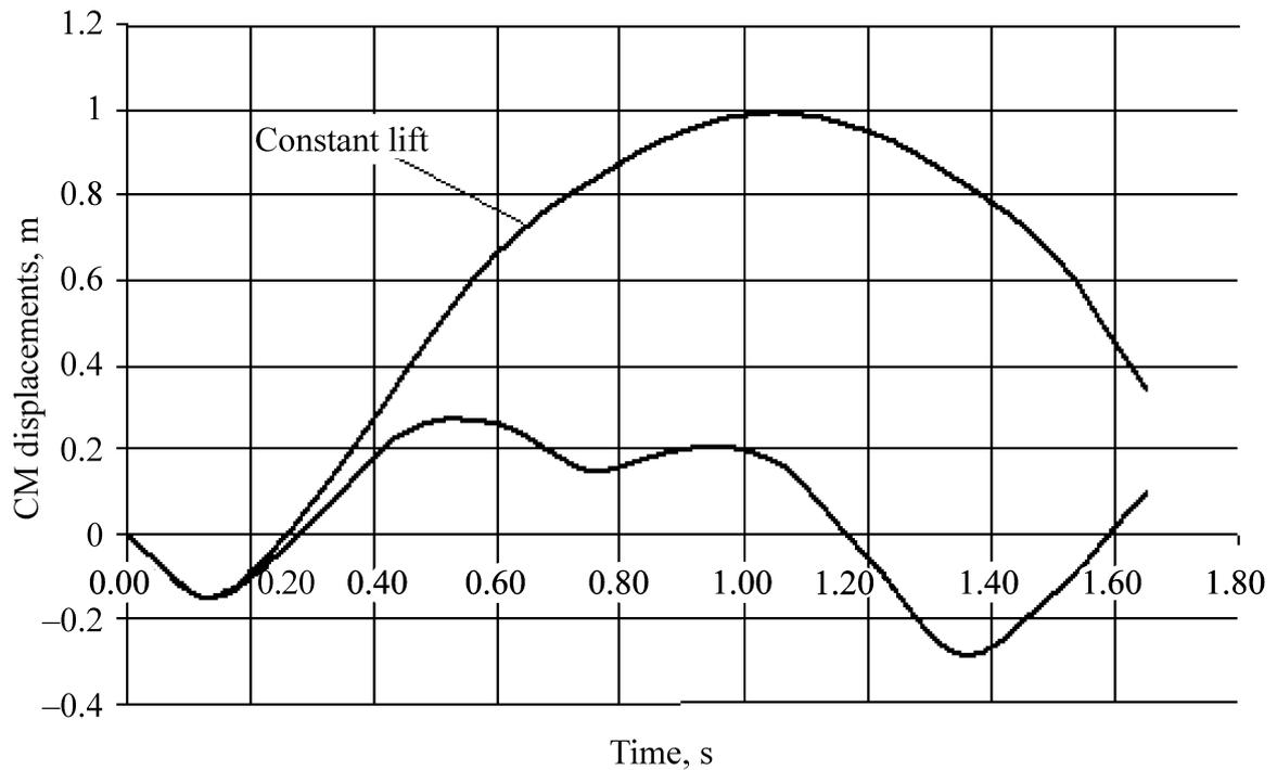
Figure 8 – Vertical Displacements of Helicopter Center of Mass in Two Variants of Rotor Lift. Initial Pitch Angle Is Equal to 5 Degrees
