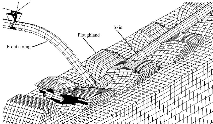
Figure 11 – Soil Deformation Behavior
