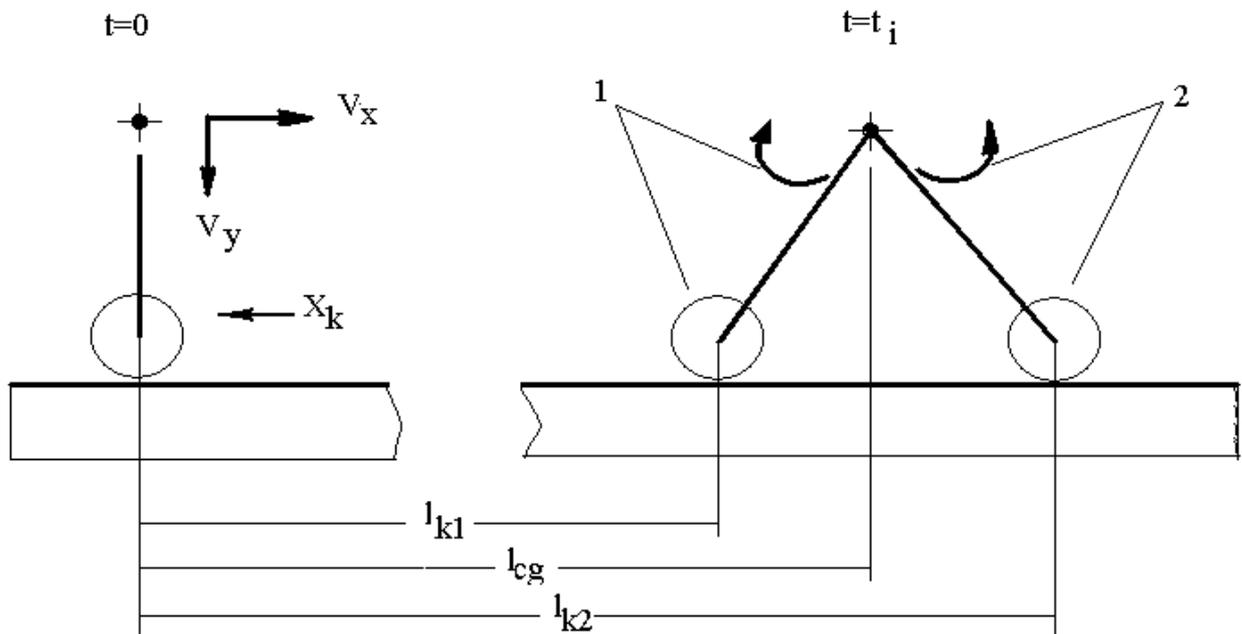
Figure 1 – Possible Positions of Helicopter LG Leg during Landing
