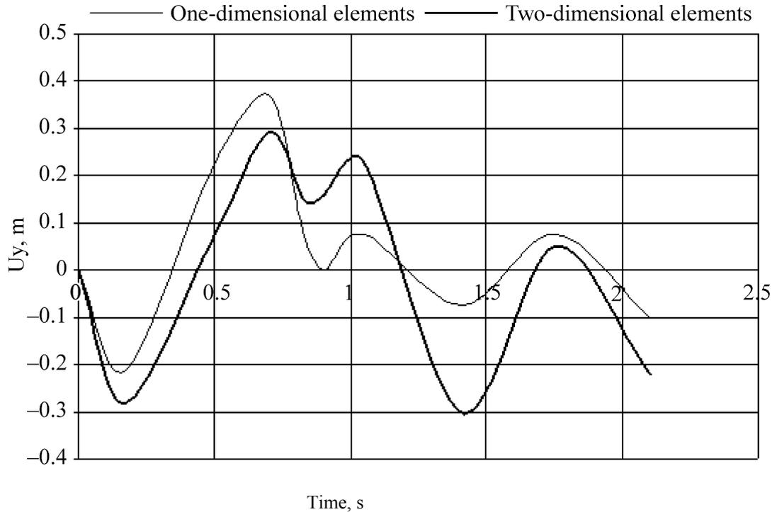
Figure 6 – Comparison of Results for One- and Two-Dimensional Skid Models
