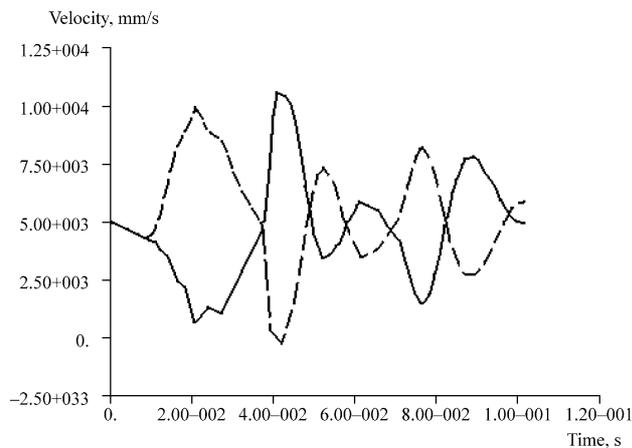
Figure 12. Spin-up of Main Landing Gear Wheels
