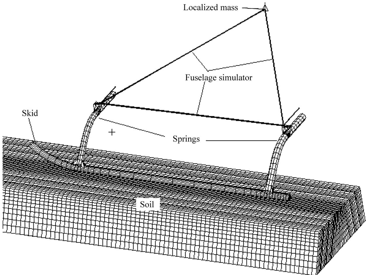
Figure 4 – Theoretical Model of Helicopter Equipped with Skid LG in Studying Off-Field Landing
