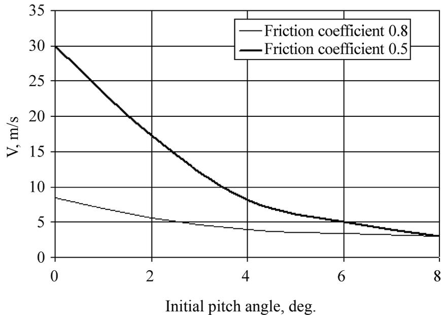
Figure 7 – Longitudinal Landing Speed Limit  $V_x$  VS Initial Pitch Angle
