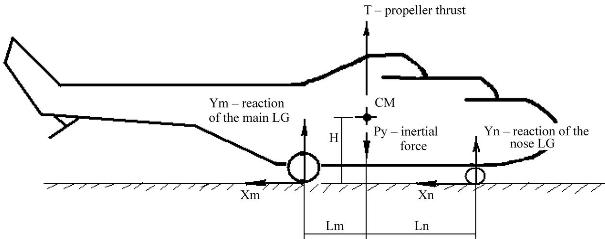
Figure 2 – System of Forces Acting on the Helicopter per FAR 29
