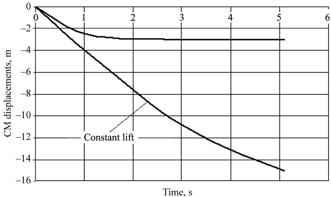
Figure 9 – Longitudinal Displacements of Helicopter Center of Mass in Two Variants of Rotor Lift. Initial Pitch Angle Is Equal to 5 Degrees
