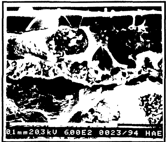
Fig. 12 - Cross-section of an HAE layer + surface sealing (varnish)
