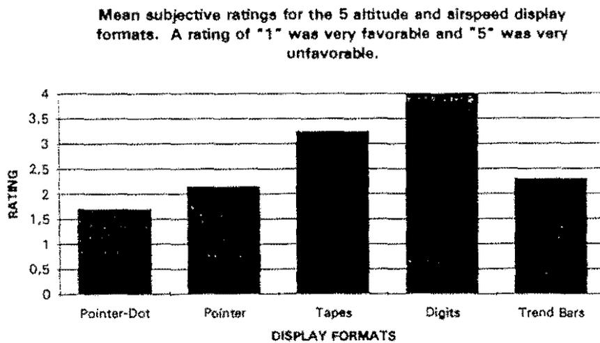
FIGURE 17. READABILITY OF DIFFERENT AIRSPEED/ALTIMETER DISPLAY
