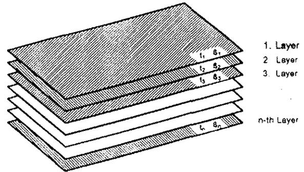
Figure 1: Geometry of general laminate
