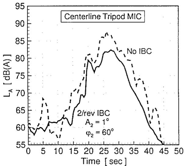
Figure 10: Noise emission as measured by the centerline tripod microphone for a 6° descent flight at 65 KIAS.
