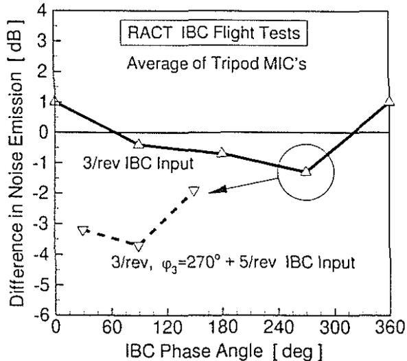
Figure 15: Influence on noise for a variation of 3/rev IBC phase angle and of 5/rev phase angle for 3/rev+5/rev IBC input.
