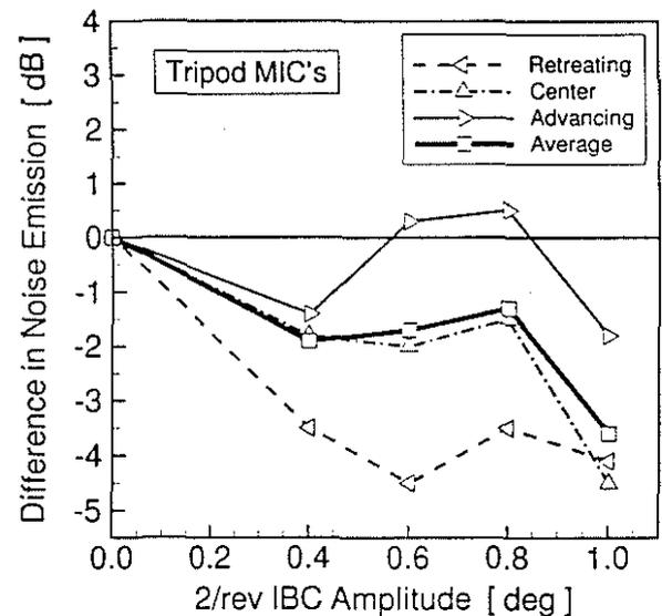
**Figure 13:** BVI noise suppression versus amplitude for a 2/rev IBC input, 60° phase angle (6° approach, 65 KIAS).
