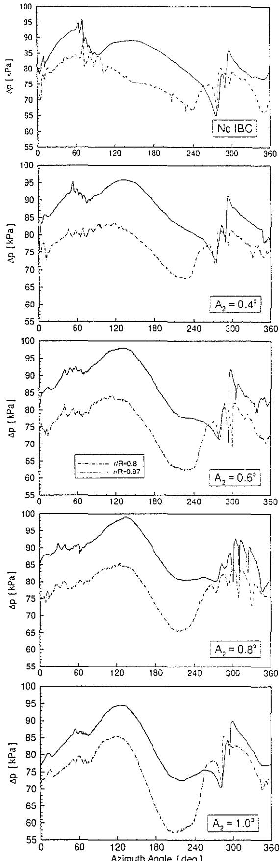
**Figure 14:** Leading edge blade pressure distribution for the 2/rev IBC amplitude sweep ( $6^\circ$  approach, 65 KIAS).
