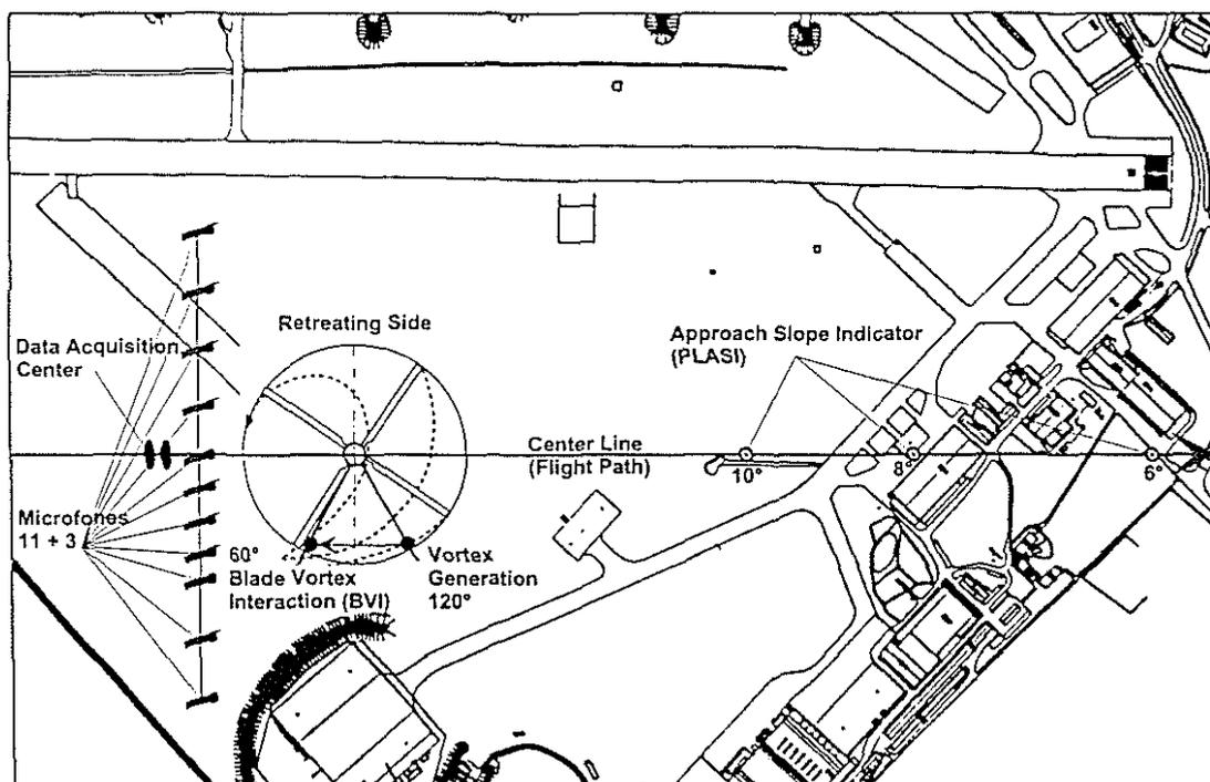
Figure 4: Arrangement of Test Equipment on Ground
