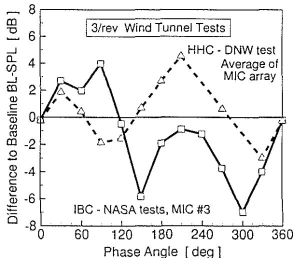
Figure 16: Results of wind tunnel tests for 3/rev HHC and IBC input for a trim condition corresponding to a  $6^\circ$  descent, 65 kts flight.
