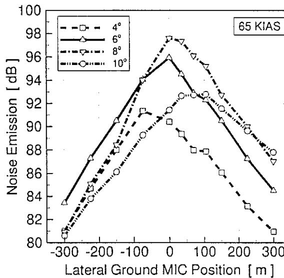
Figure 5: Noise emission for various approach slope angles at 65 KIAS, IBC not activated.
