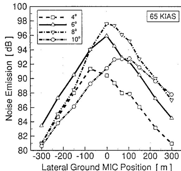
**Figure 5:** Noise emission for various approach slope angles at 65 KIAS, IBC not activated.
