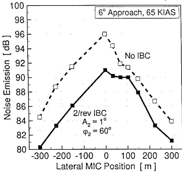
Figure 9: Noise emission as measured by the ground-based microphone array for a 6° descent flight at 65 KIAS.
