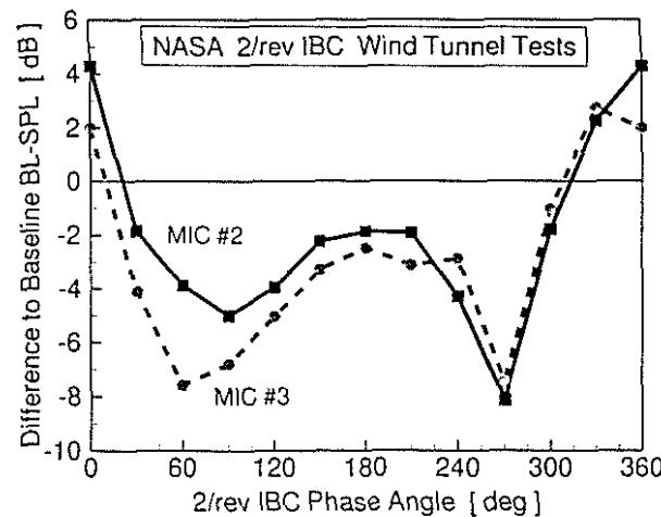
[Figure 7:](#) BVI noise reduction versus phase angle for a 2/rev, 1° amplitude IBC input as measured in the NASA wind tunnel.
