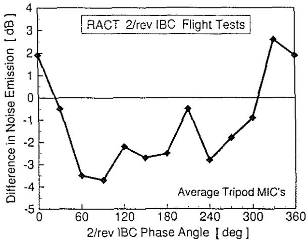
**Figure 6:** BVI noise reduction versus phase angle for a 2/rev, 1° amplitude IBC input as measured in the RACT flight tests.
