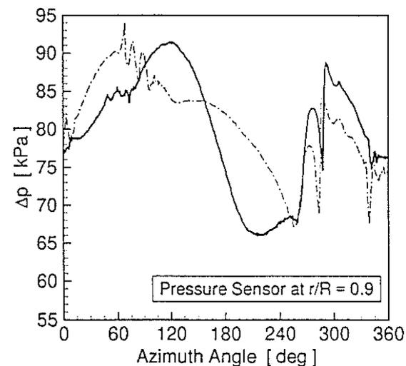
Figure 11: Leading edge blade pressure distribution versus azimuth angle for three radial stations (6° approach, 65 KIAS).
