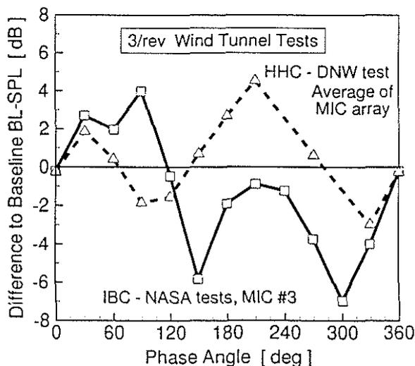
Figure 16: Results of wind tunnel tests for 3/rev HHC and IBC input for a trim condition corresponding to a 6° descent, 65 kts flight.
