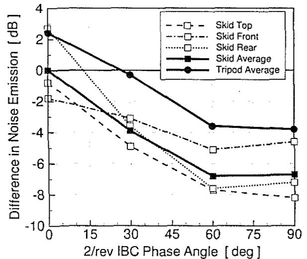
**Figure 8:** Noise reduction versus phase angle as measured by the landing skid microphones, 2/rev IBC input, 1° amplitude, 6° descent flight at 65 KIAS.
