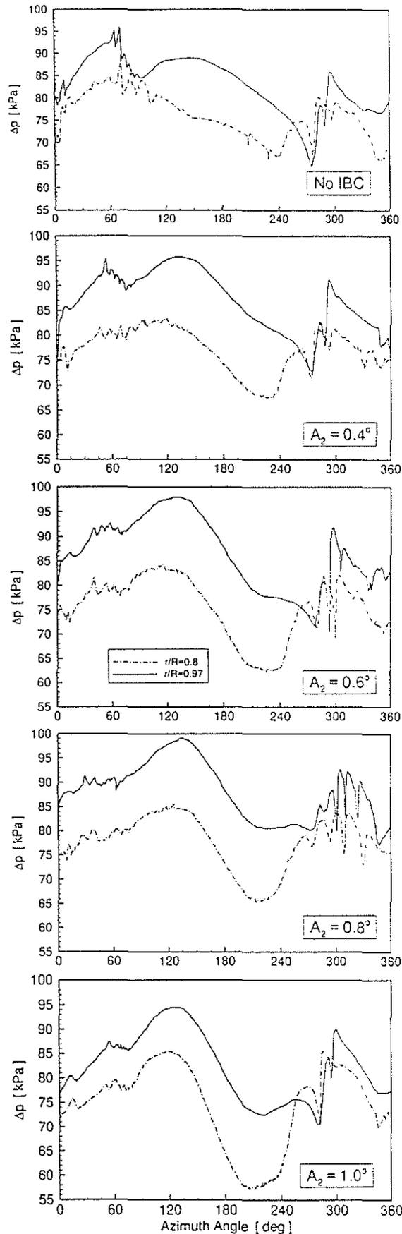
Figure 14: Leading edge blade pressure distribution for the 2/rev IBC amplitude sweep (6° approach, 65 KIAS).
