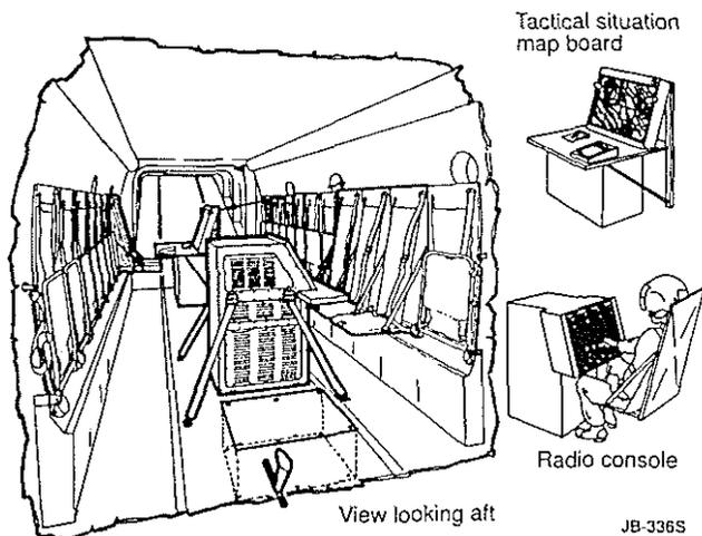
Figure 21. V-22 Command and Control Cabin
