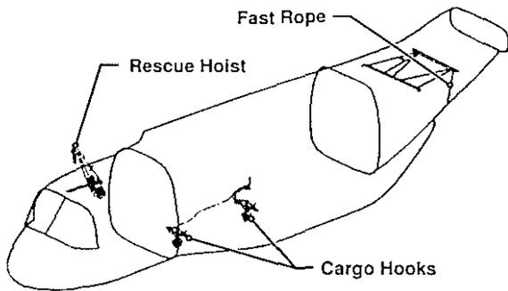
Figure 12. External Load Handling Equipment
