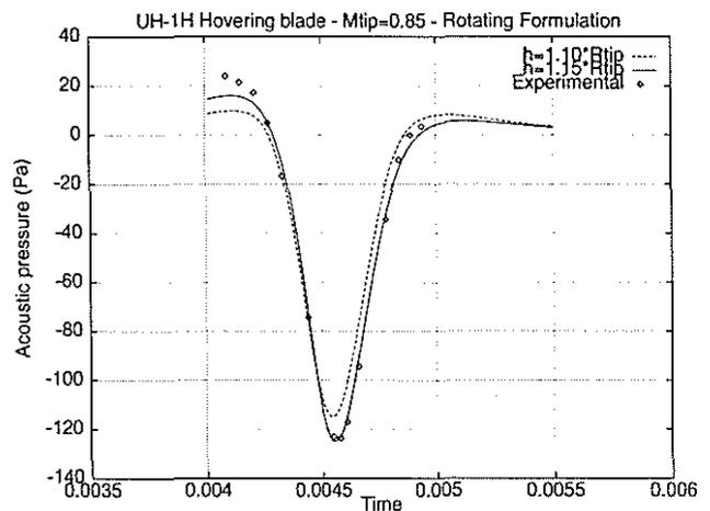
Figure 20: Aeroacoustic pressure at  $M_{tip} = 0.85$  as a function of the height of the Kirchhoff surface
