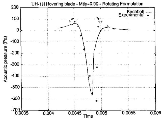
Figure 24: Aeroacoustic pressure at  $M_{tip} = 0.90$  - limiting the integration inside the sonic circle
