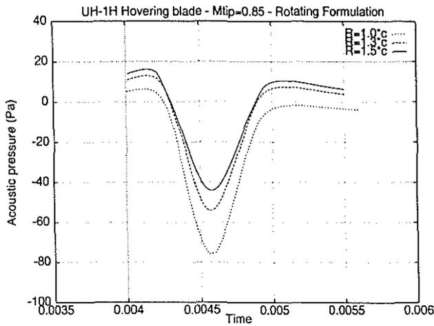
Figure 22: Aeroacoustic pressure at  $M_{tip} = 0.85$  - Lateral surface contribution
