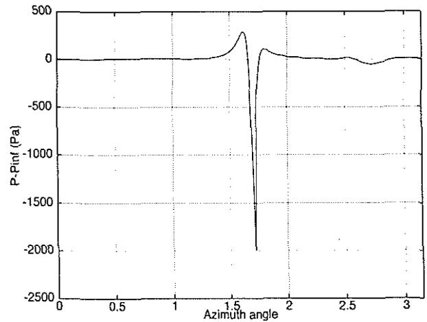
Figure 5: Input pressure distribution on the Kirchhoff cylinder in the rotor plane at  $M_{tip} = 0.90$
