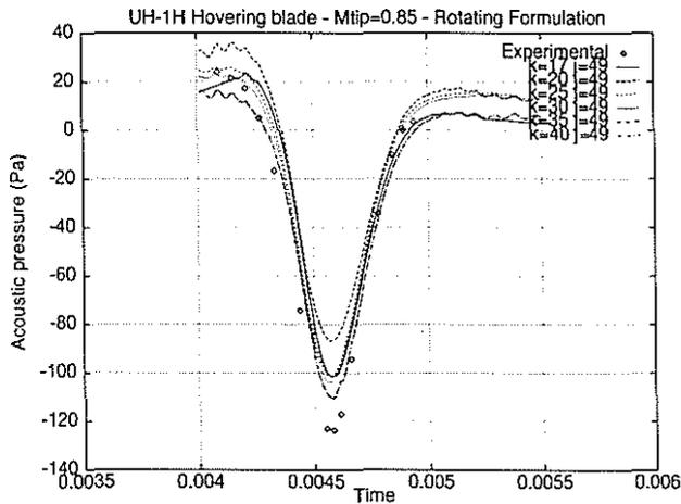
Figure 18: Comparison of aeroacoustic pressure computed at  $M_{tip} = 0.85$  using k-constant layers of the aerodynamic mesh - 49 span stations -
