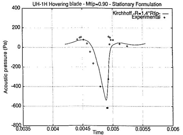
Figure 9: Aeroacoustic pressure at  $M_{tip} = 0.90$
