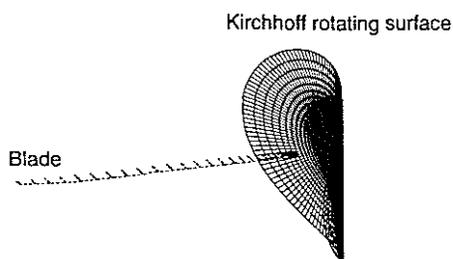
Figure 16: Kirchhoff surface directly extracted from the aerodynamic mesh with a constant span index
