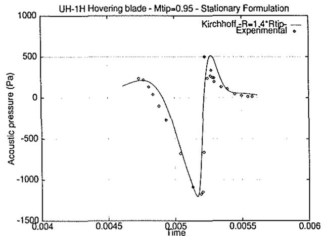
Figure 12: Aeroacoustic pressure at  $M_{tip} = 0.95$
