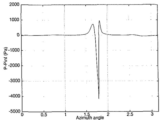
Figure 6: Input pressure distribution on the Kirchhoff cylinder in the rotor plane at  $M_{tip} = 0.95$
