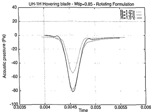
Figure 23: Aeroacoustic pressure at  $M_{tip} = 0.85$  - Base end surface contribution
