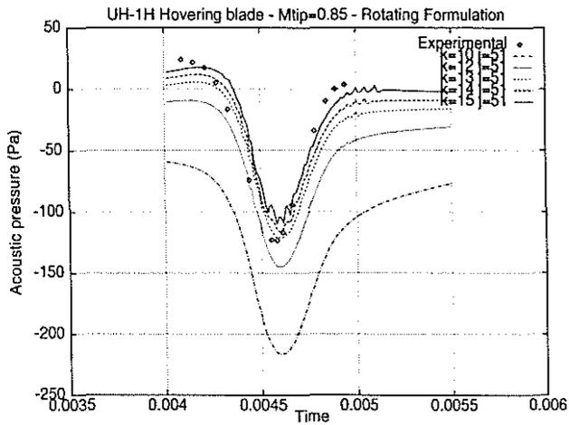
Figure 17: Comparison of aeroacoustic pressure computed at  $M_{tip} = 0.85$  using k-constant layers of the aerodynamic mesh - 51 span stations -
