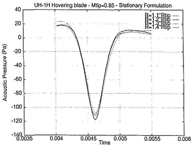
Figure 8: Pressure signal as a function of the radial position of the Kirchhoff surface at  $M_{tip} = 0.85$
