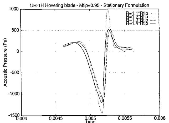
Figure 14: Pressure signal as a function of the radial position of the Kirchhoff surface at  $M_{tip} = 0.95$
