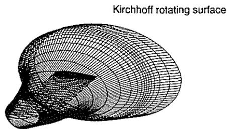
Figure 15: Kirchhoff surface directly extracted from the aerodynamic mesh with a constant vertical index
