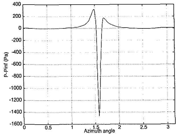
Figure 4: Input pressure distribution on the Kirchhoff cylinder in the rotor plane at  $M_{tip} = 0.85$
