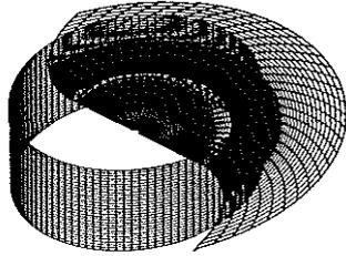
Figure 3: Z-constant plane of Euler grid and Kirchhoff cylinder
