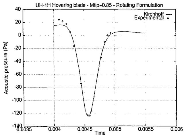
Figure 19: Aeroacoustic pressure at  $M_{tip} = 0.85$
