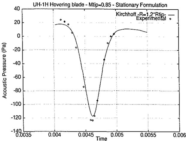
Figure 7: Aeroacoustic Pressure at  $M_{tip} = 0.85$
