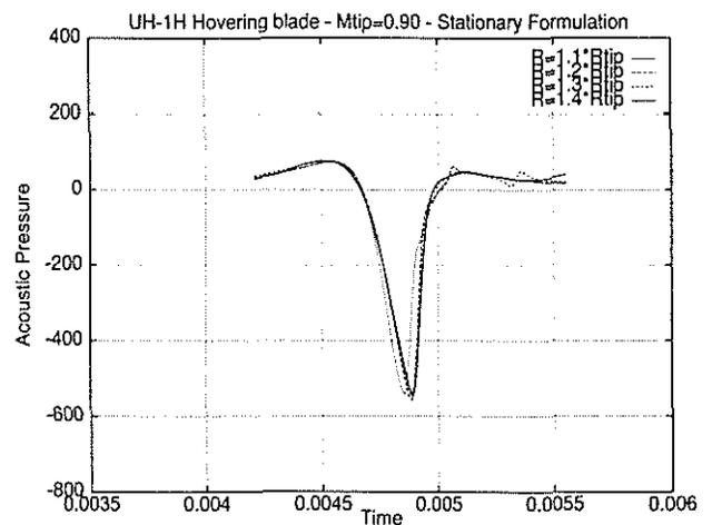
Figure 11: Pressure signal as a function of the radial position of the Kirchhoff surface at  $M_{tip} = 0.90$
