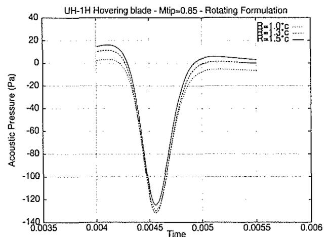
Figure 21: Aeroacoustic pressure at  $M_{tip} = 0.85$  as a function of the radius of the Kirchhoff surface
