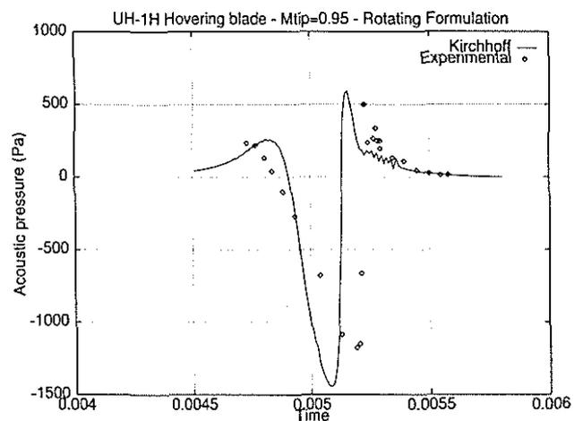
Figure 25: Aeroacoustic pressure at  $M_{tip} = 0.95$  - limiting the integration inside the sonic circle
