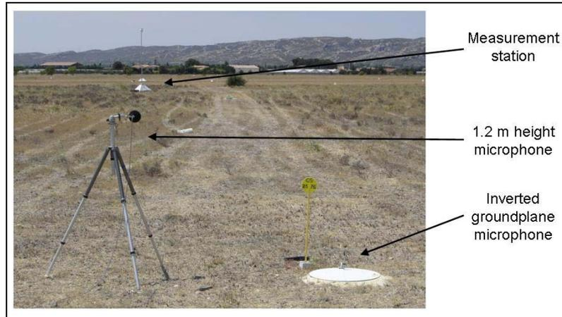
Figure 5. Microphone installation, showing 1.2m-height and ground plane microphones
