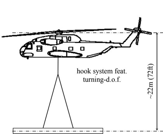
Figure 5: Helicopter slung load configuration
