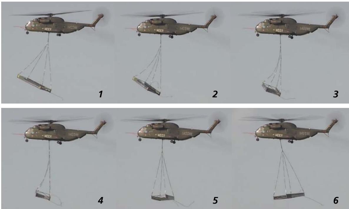
Figure 13: Image series of cable bounce due to load aerodynamic activity at 20 KIAS
