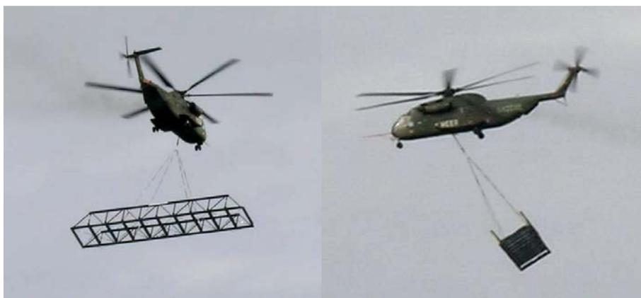
Figure 9: Bridge 1 at 50 KIAS forward flight
