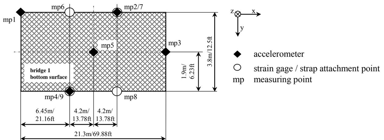
Figure 1: Sketch of measuring points at bridge 1
