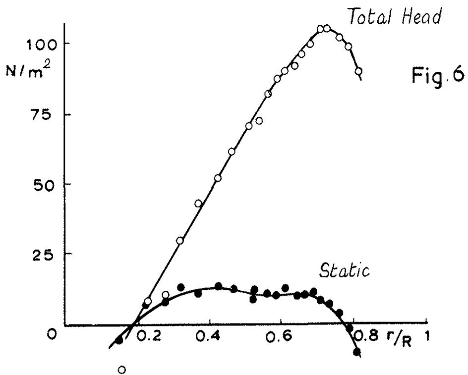
Figs. 5 & 6 Pressure Distributions (Rotor B)
