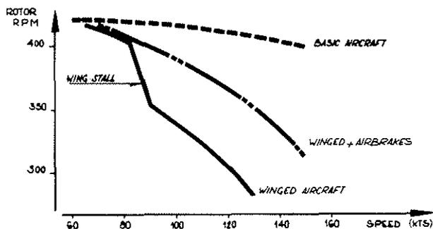
Fig 5: EFFECT OF WING AND AIRBRAKES ON ROTOR RPM IN AUTOROTATION
