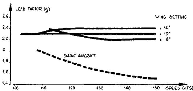
FIG 2: MAXIMUM LOAD FACTOR AT CONSTANT COLLECTIVE PITCH (13°)
