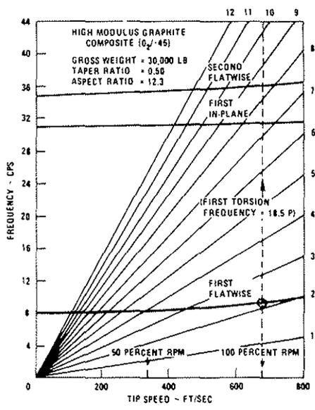
Figure 17 - X-Wing Rotor Blade Frequency Characteristics
