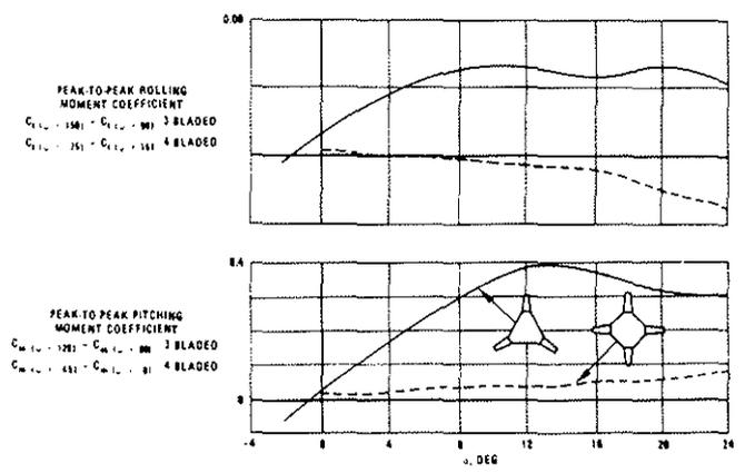
Figure 18 - Effect of Four Blades on the Reduction of Peak-to-Peak Moments during the Rotor Revolution (Reference 5)
