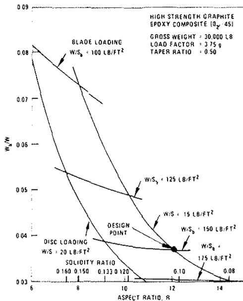
Figure 13a – Blade Weight/Gross Weight Ratio
