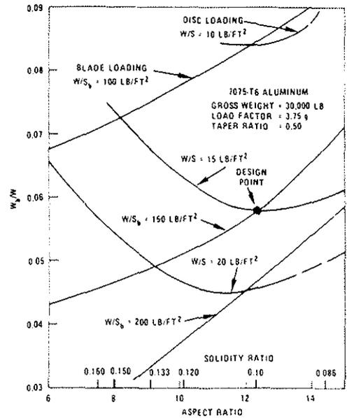
Figure 12a – Blade Weight/Gross Weight Ratio
