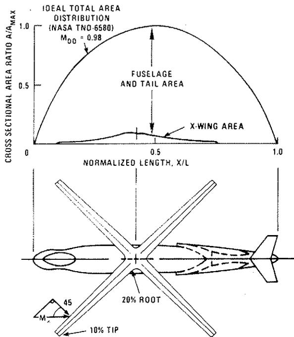
Figure 3 - X-Wing Transonic Design Features (Approximate Drag Divergence Mach = 0.89)
