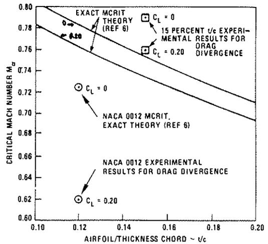
Figure 2 - Compressibility Characteristics of Two Dimensional C.C. Airfoils at Zero Angle of Attack
