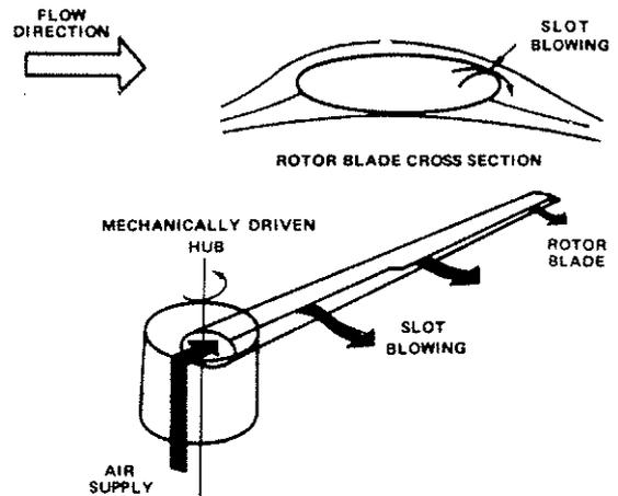
Figure 4 - Circulation Control Rotor-Basic Concept
