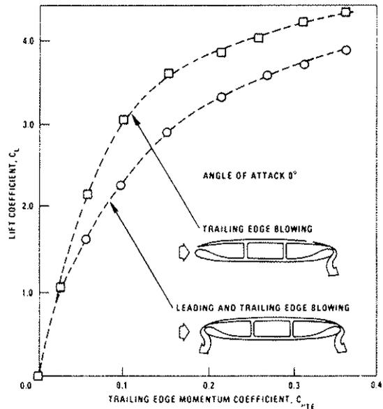
Figure 6 - Effect of Simultaneous Leading and Trailing Edge Blowing
