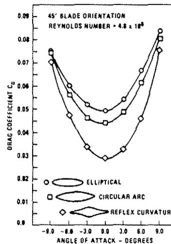
Figure 10 - Drag Coefficient (Based on Hub Planform Area) for Three Hubs with Shanks
