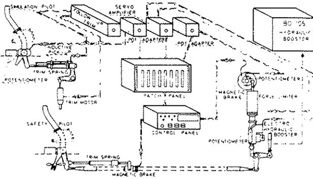
Figure 6: Fly-by-wire system of the BO 105 in-flight simulator.
