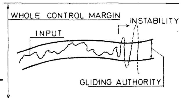
Figure 10: Authority limits of the BO 105 in-flight simulator.
