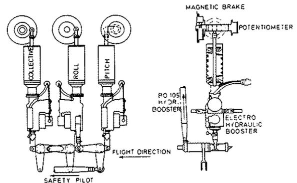
Figure 8: BO 105 in-flight simulator; connection of fly-by-wire and mechanical system.
