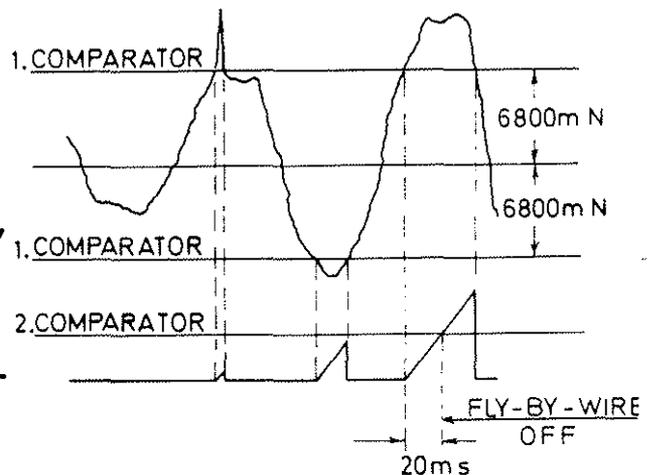
Figure 9: Monitoring of shaft moment of the BO 105 in-flight-simulator.
