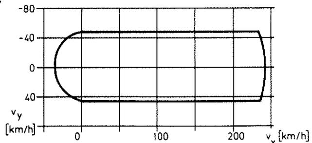
**Figure 2:** Horizontal velocity limits of the BO 105 in-flight simulator
