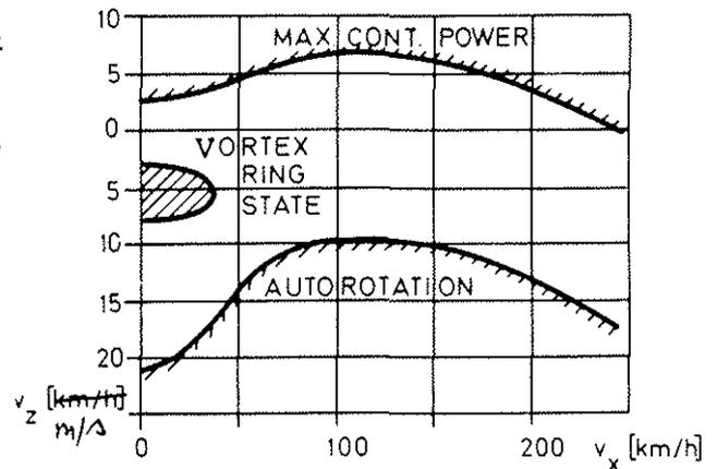
Figure 3: Vertical velocity limits of the BO 105 versus forward velocity
