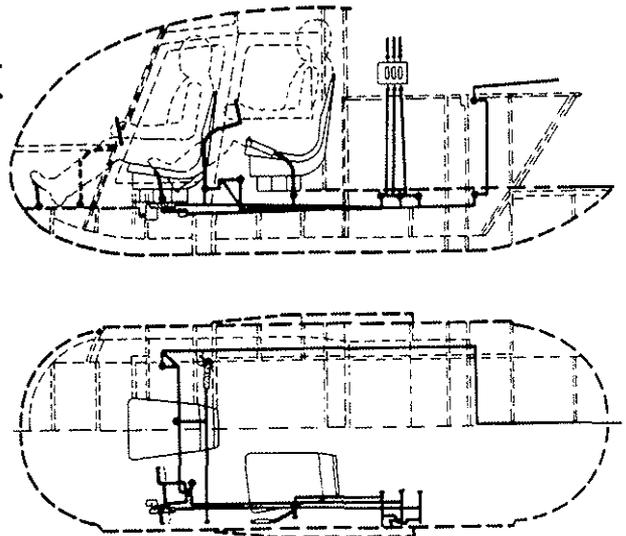
Figure 4: Design of cockpit and mechanical control system of the BO 105 in-flight simulator.
