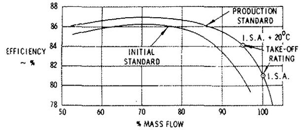
Fig. 17 L.P. Compressor Operating Line Efficiency
