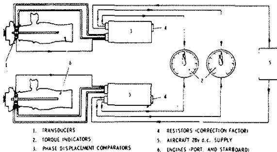
Fig. 14 Torquemeter System Diagram (2 Engines)
