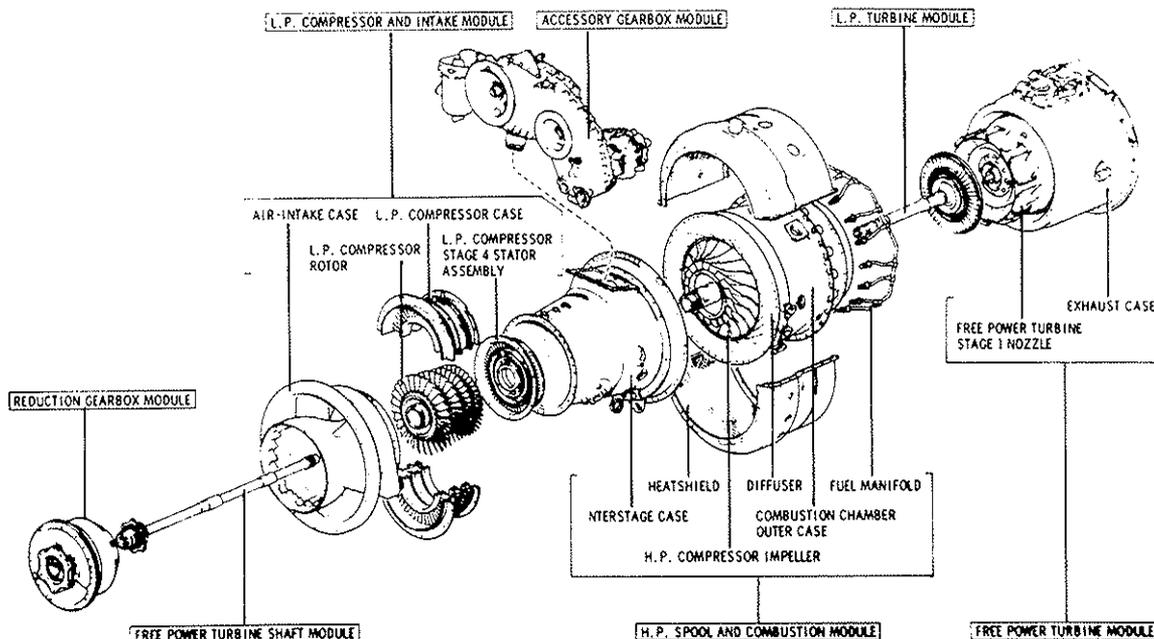
Fig. 9 Gem Engine Modules
