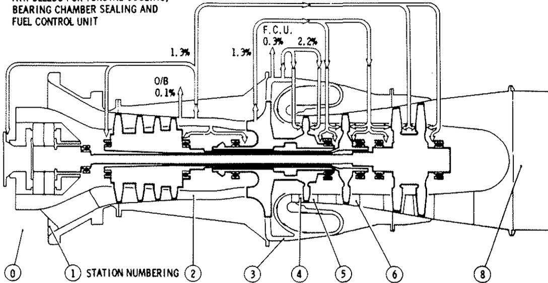
**Fig. 18 Bearings and Air System**
