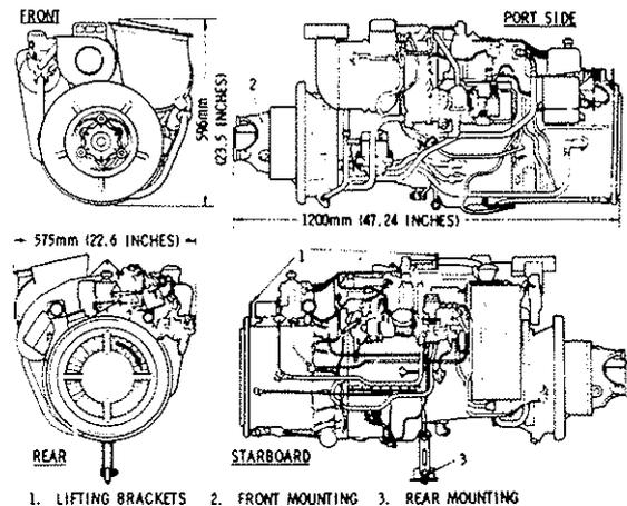
Fig. 6 Gem Installation Diagram
