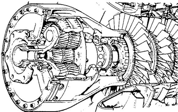
Fig. 11 Main Reduction Gearbox
