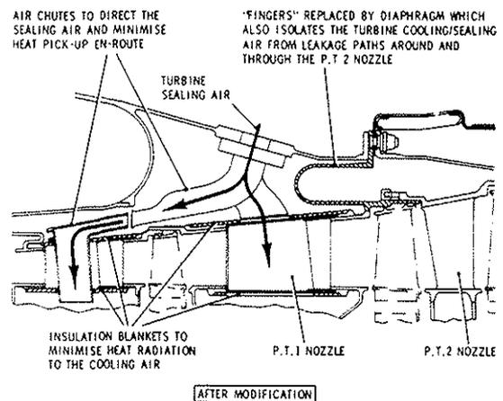
**Fig. 19 Gem Turbine Cooling Arrangement**
