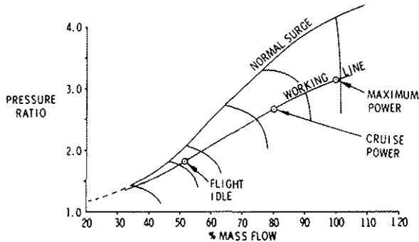
Fig. 15 L.P. Compressor Characteristics and Operating Line
