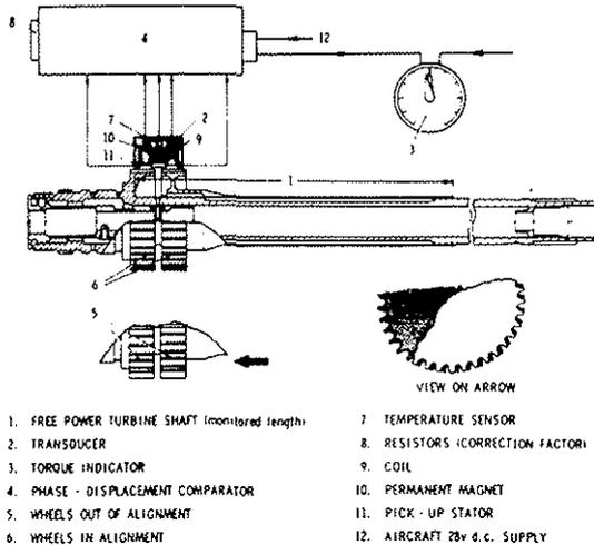
Fig. 13 Torquemeter Operation (1 Engine)
