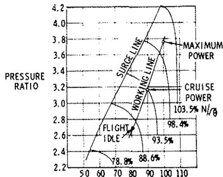
Fig. 16 H.P. Compressor Operating Line Efficiency
