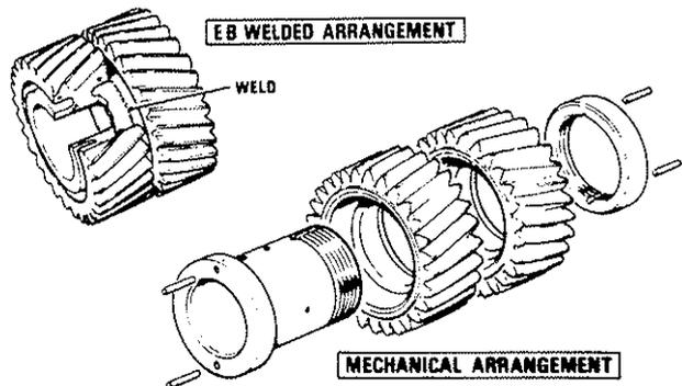
Fig. 12 Planet Pin Construction
