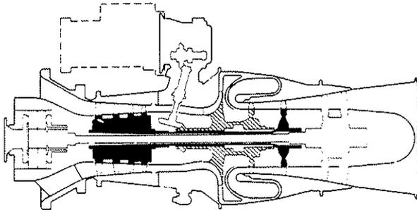
Fig. 7 Gem Two-Spool Turboshaft
