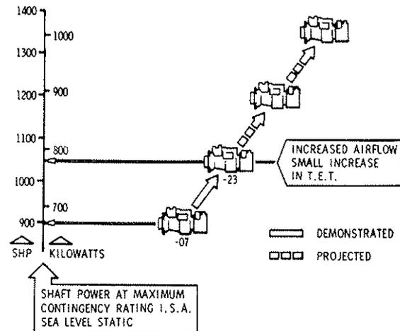
Fig. 20 Up-rating Diagram
