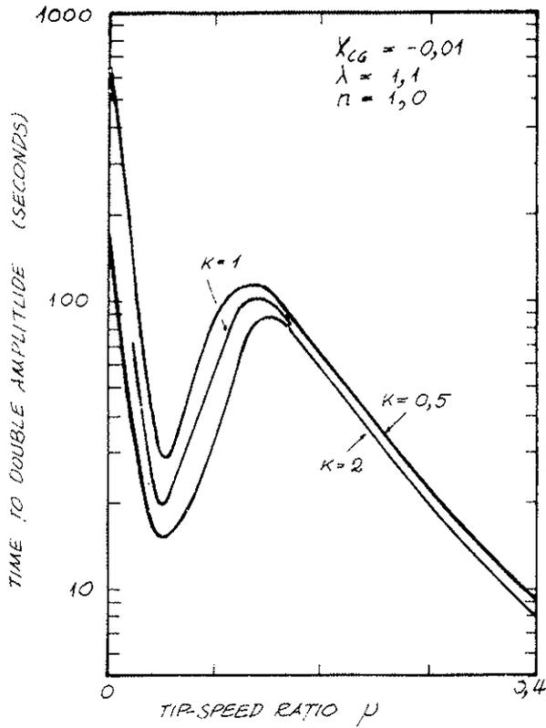
FIG. 8 STABILITY WITH A DISC-TILT DEMAND CONTROL SYSTEM
