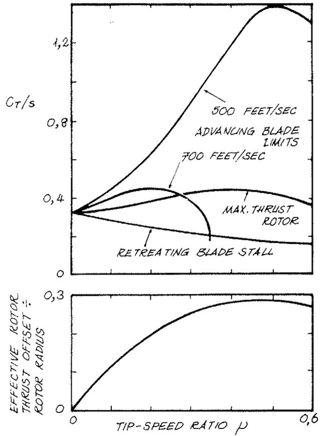
FIG. 9 ROTOR THRUST LIMITS
