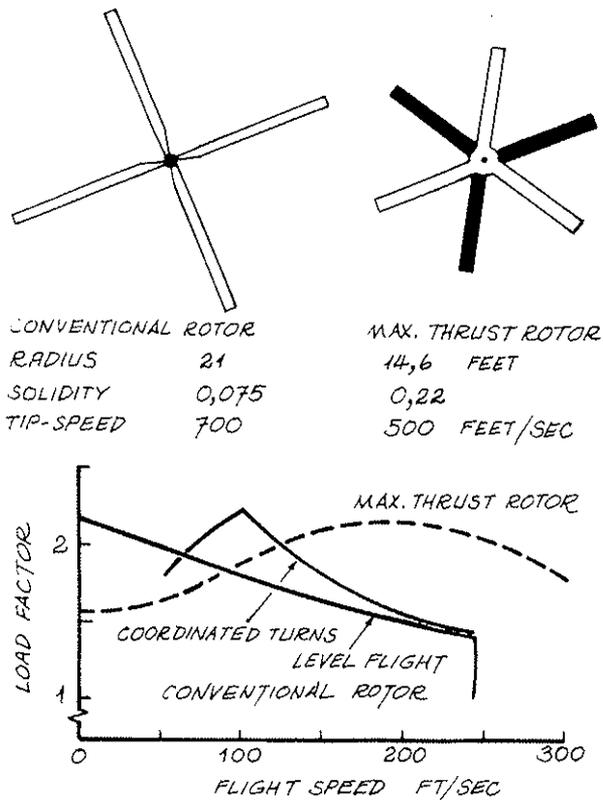
FIG. 10 COMPARISON OF CONVENTIONAL AND MAXIMUM-THRUST ROTORS
