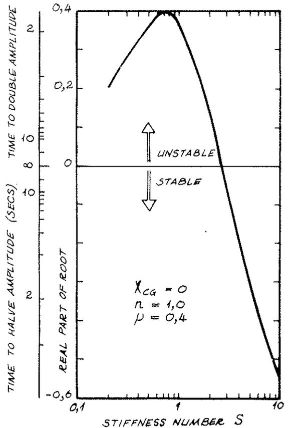
FIG. 11 EFFECT OF HIGH STIFFNESS ON HELICOPTER STABILITY
