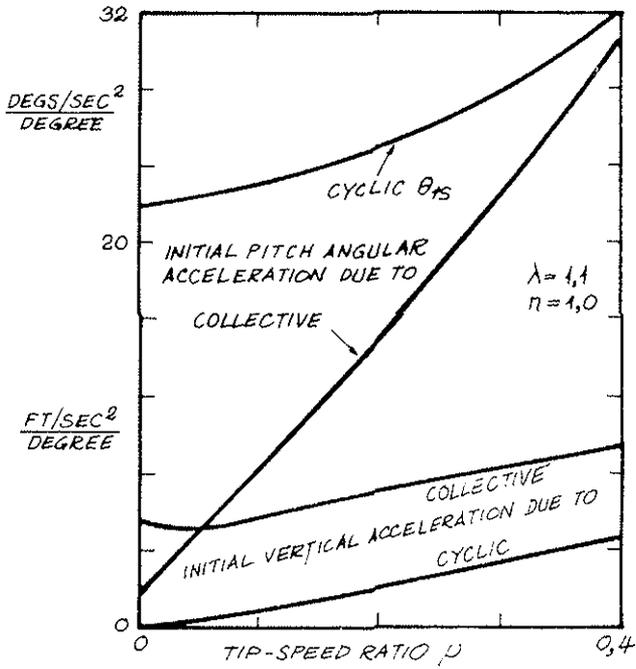
FIG. 4 ROTOR CONTROL COUPLING
