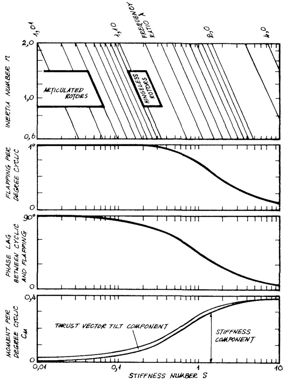
FIG. 2 HELICOPTER ROTOR CHARACTERISTICS
