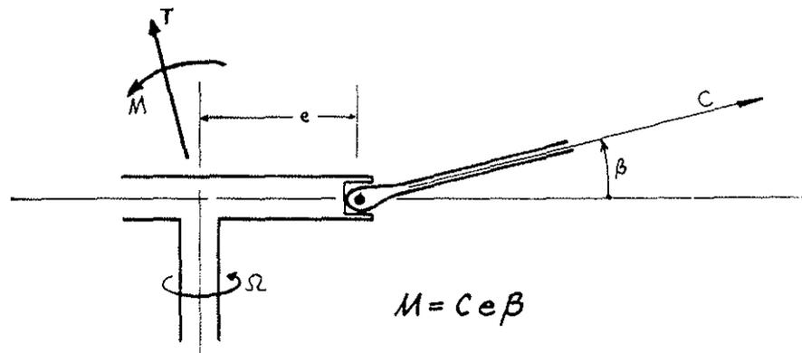
FIG.1 THE ARTICULATED ROTOR
