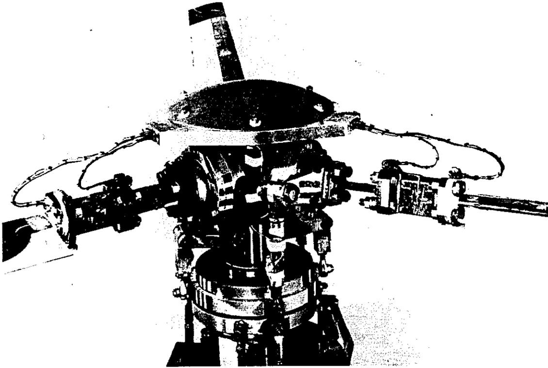
Fig.3 Rotor head
