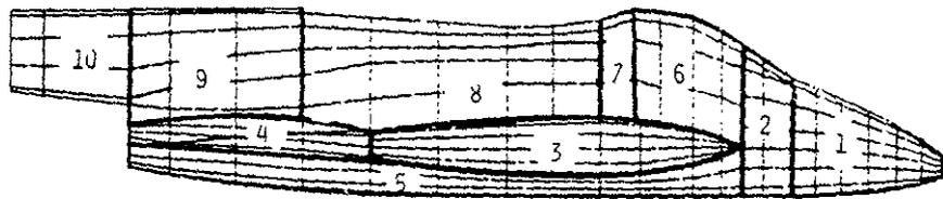
Fig. 9. Typical Example of Multi-Patch Body Paneling.
