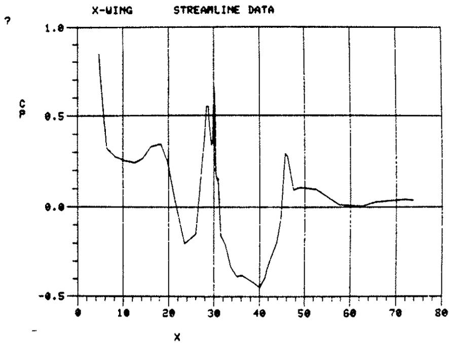
Fig. 22. Typical Streamline Output Data Plot. X-Wing Top Centerline Potential Flow Streamline.
