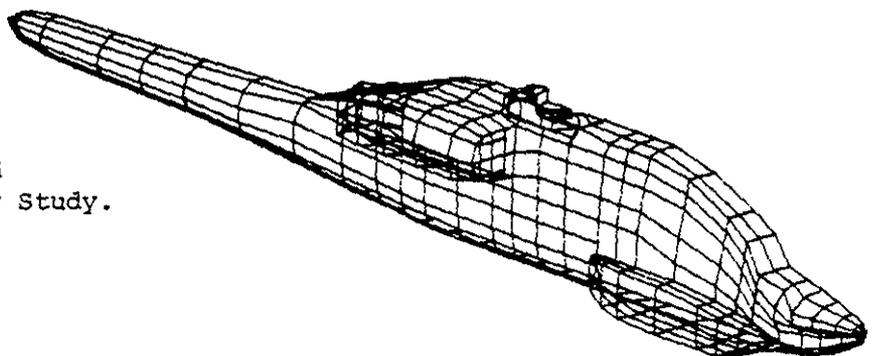
Fig. 11. Baseline Attack Helicopter Panelled for Hub/Pylon Drag Study.
