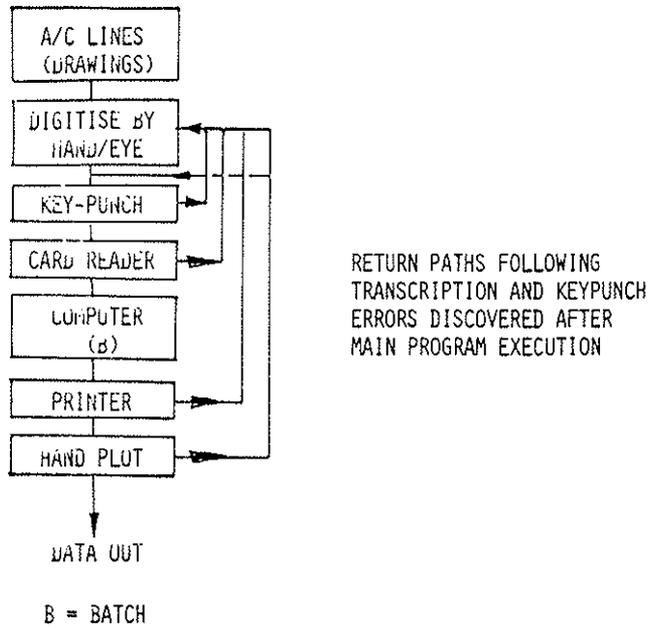
Fig. 15. Block Diagram for Serial Operation of an Involved Batch Mode Computer Program.
