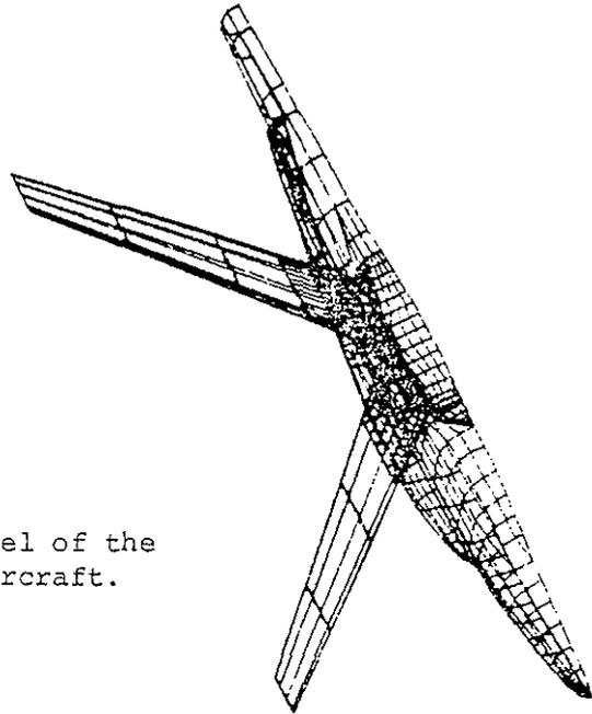
Fig. 13. Panel Model of the X-Wing Aircraft.
