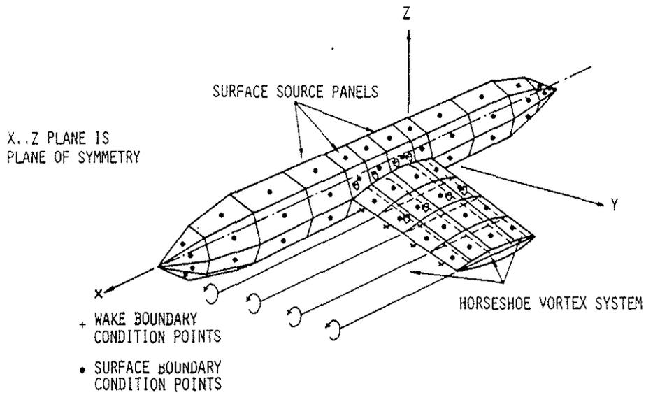
Fig. 1. Schematic of Source and Vortex Panel Potential Flow Model.
