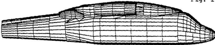
Fig. 10. Baseline Utility Transport Helicopter Panelled for Hub/Pylon Drag Study.
