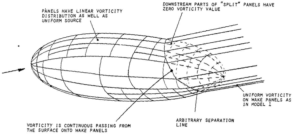
Fig. 8. Schematic of Program DRAG Model.
