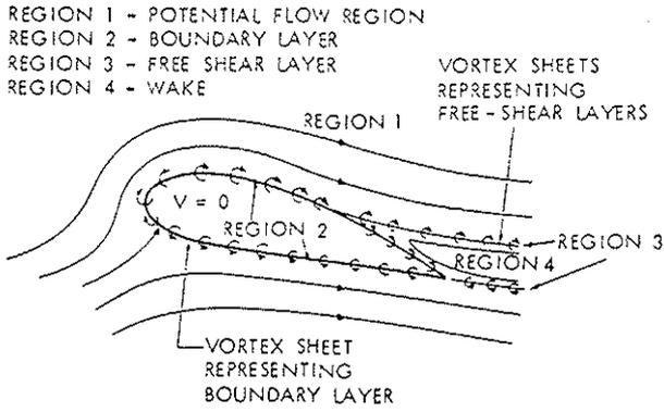
Fig. 4. Improved Model of Separated Flow Region Used in CLMAX Program.
