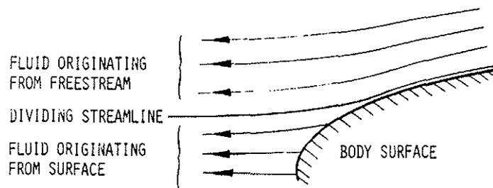
Fig. 2. Modeling of Potential Flow to Account for Separated Regions.
