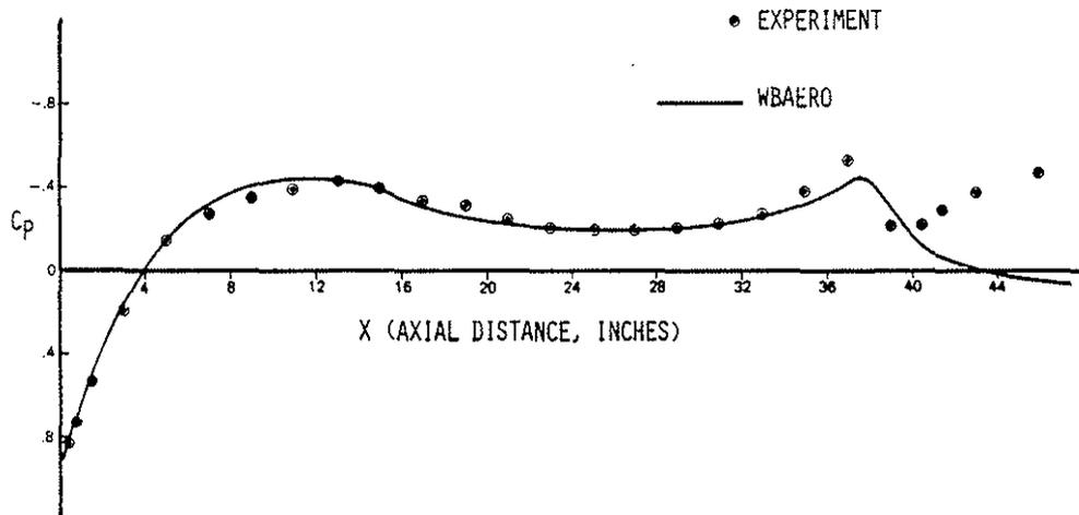
Fig. 3. Pressure Distribution Along Top Centerline of B0105 Calculated Using WBAERO.  $0^\circ$  Pitch,  $10^\circ$  Yaw.
