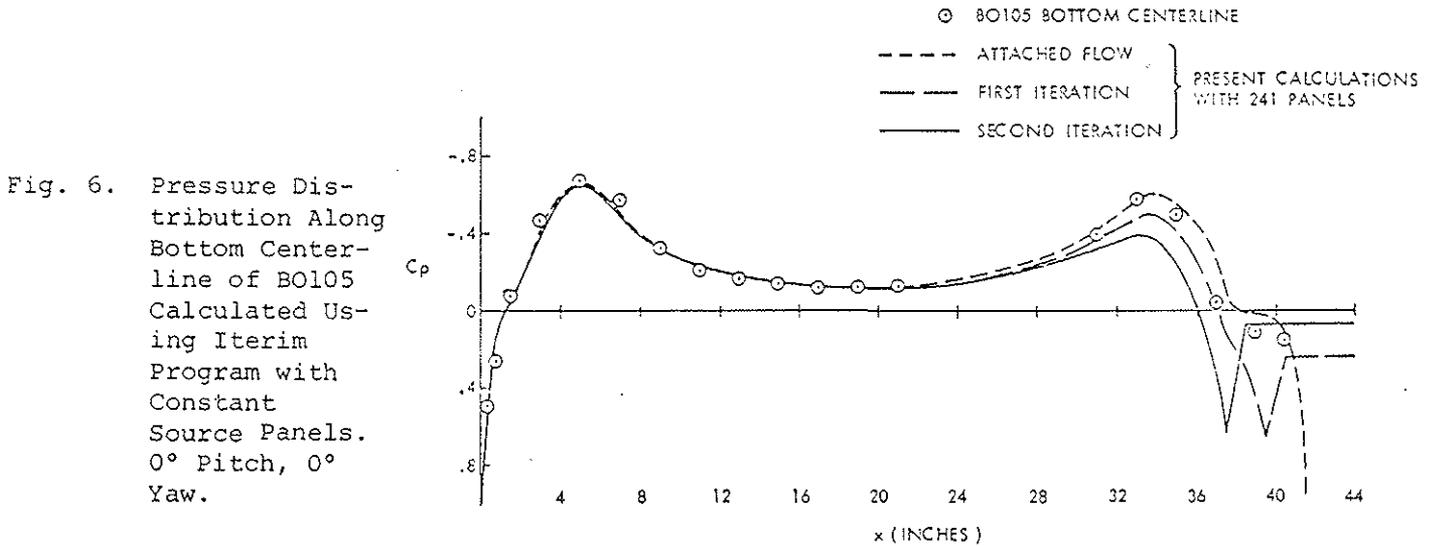
Fig. 6. Pressure Distribution Along Bottom Centerline of BO105 Calculated Using Iterim Program with Constant Source Panels.  $0^\circ$  Pitch,  $0^\circ$  Yaw.
