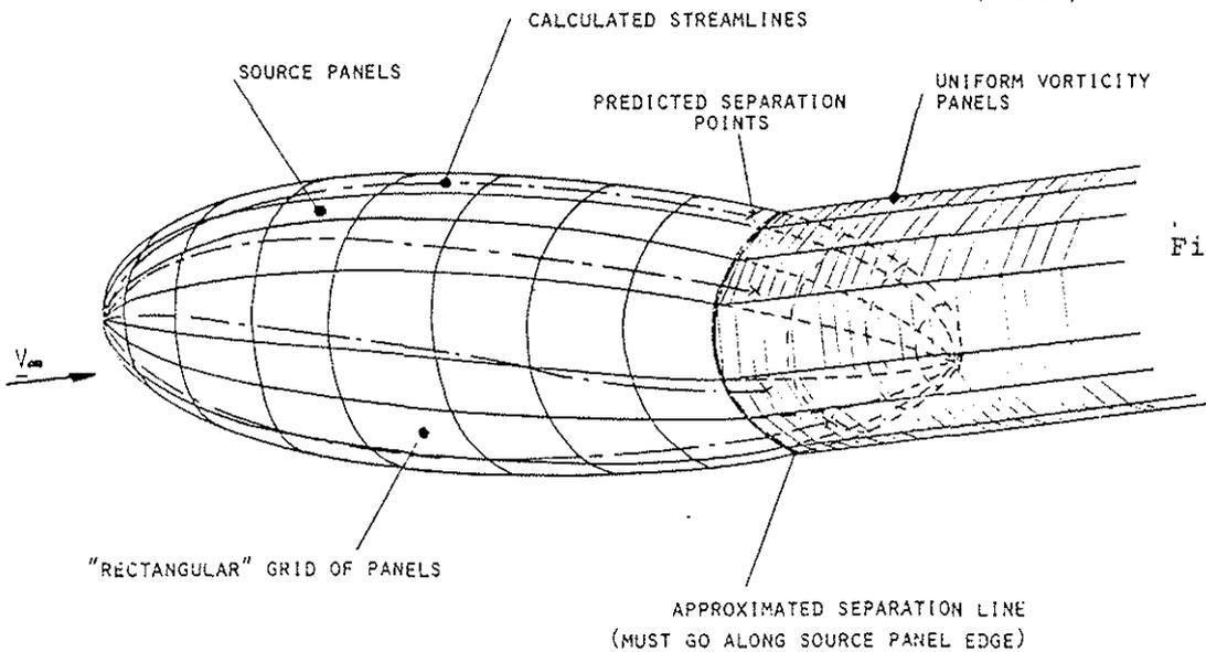
Fig. 7. Schematic of Interim Model for Modeling Separated Flow on Bodies.
