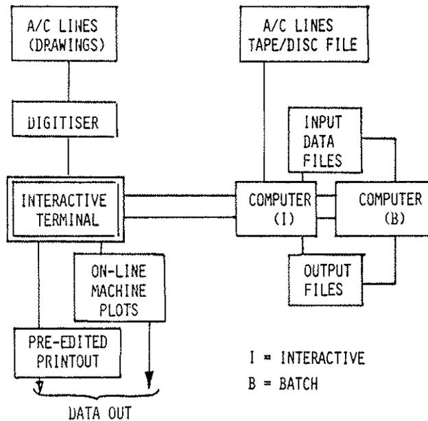
Fig. 16. Block Diagram of the Interactive Operation of Involved Configuration Modeling Programs.
