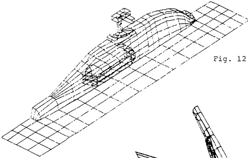
Fig. 12. Partial Attack Helicopter Model on Wind Tunnel Ground Plane.
