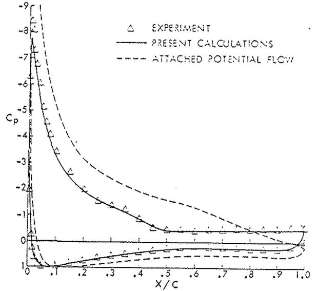
Fig. 5. Typical Correlation of Post Stall Airfoil Pressure Distribution Using CLMAX Program.
