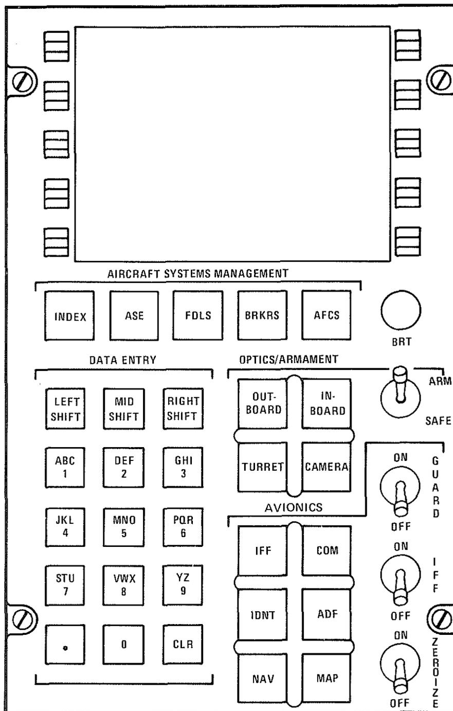
Figure 4: Control and Display Unit
