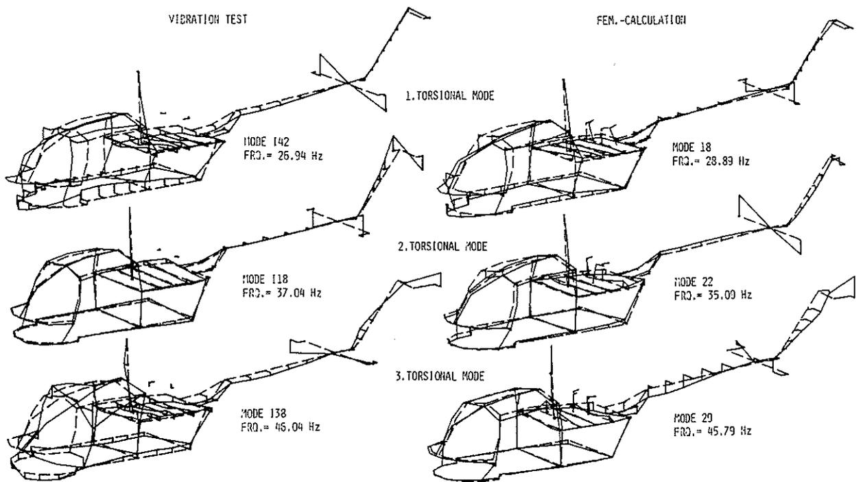
Figure 12: Torsional modes of fuselage of helicopter BO 105, comparison vibration test - fem.-calculation
