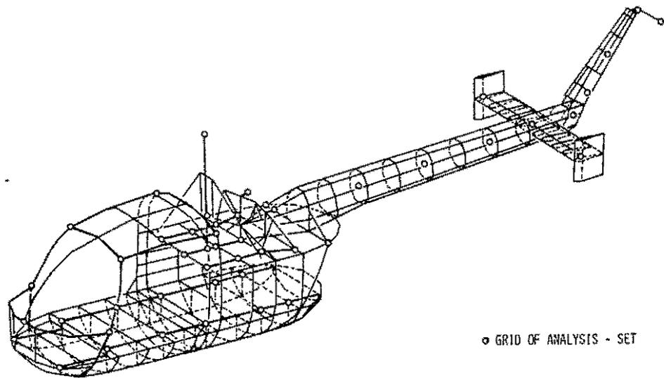
Figure 2: Analysis - set of model of helicopter BO 105
