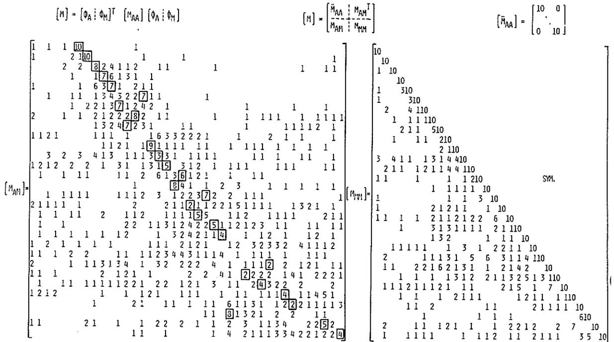
Figure 8: Generalized mass matrix (normalized to 10)
