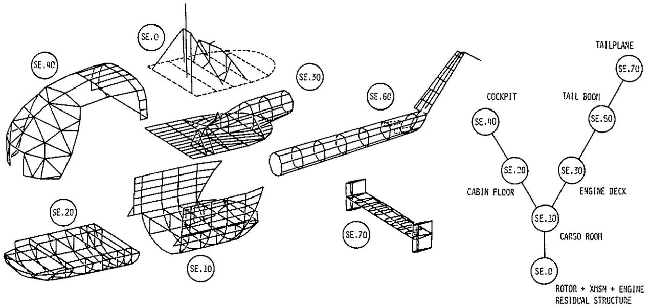
Figure 3: Idealisation of helicopter BO 105, multi - level - substructuring
