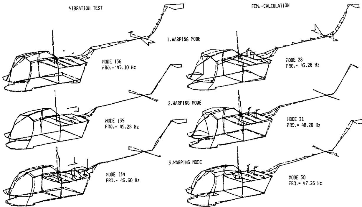
Figure 14: Warping modes of engine deck of helicopter BO 105, comparison vibration test - fem.-calculation
