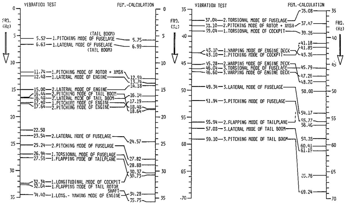
Figure 9: Natural frequencies and modes of helicopter BO 105, comparison vibration test - fem.-calculation
