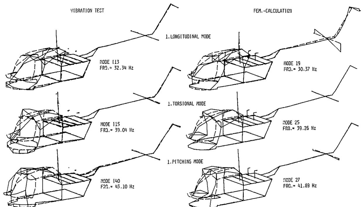
Figure 13: Natural modes of cockpit of helicopter BO 105, comparison vibration test - fem.-calculation
