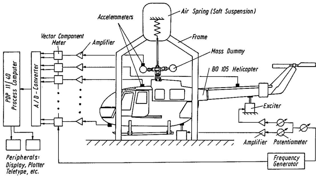
Figure 5: Diagrammatic test setup
