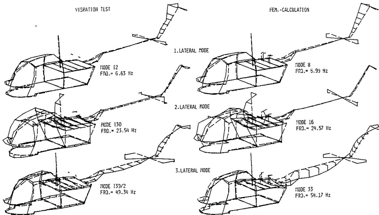
Figure 10: Lateral modes of fuselage of helicopter BO 105, comparison vibration test - fem.-calculation
