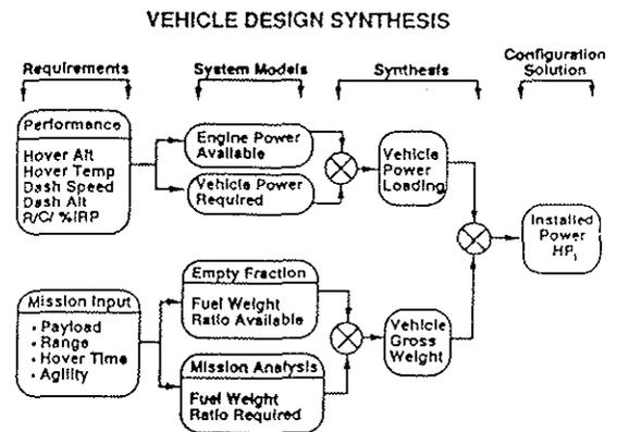
Fig. 1 Vehicle Design Synthesis
