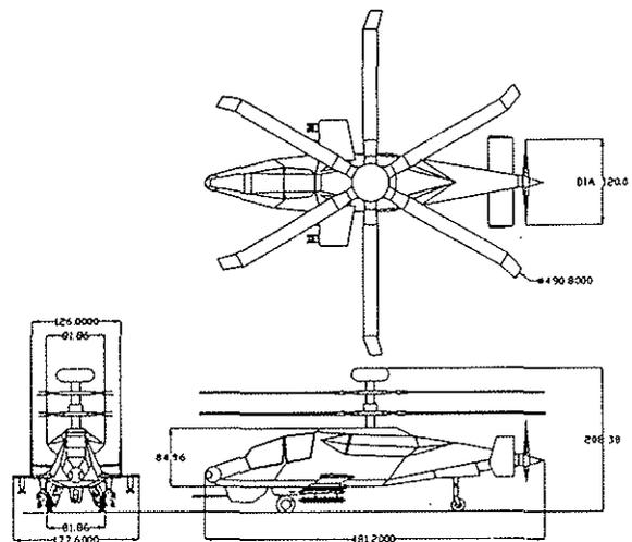
**Fig. 10 A Coaxial Compound HSHMR 3 View Drawings**
