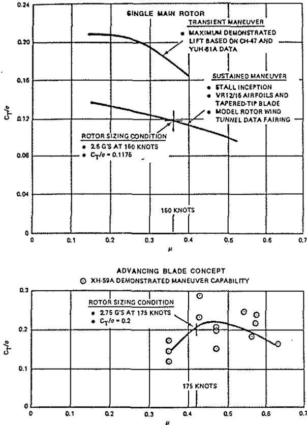
Fig. 9 Maneuver Rotor Lift Boundaries
