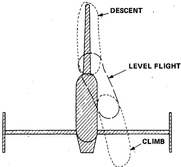
Figure 4: ROTOR HEAD WAKE POSITION RELATIVE TO TAIL SURFACES
