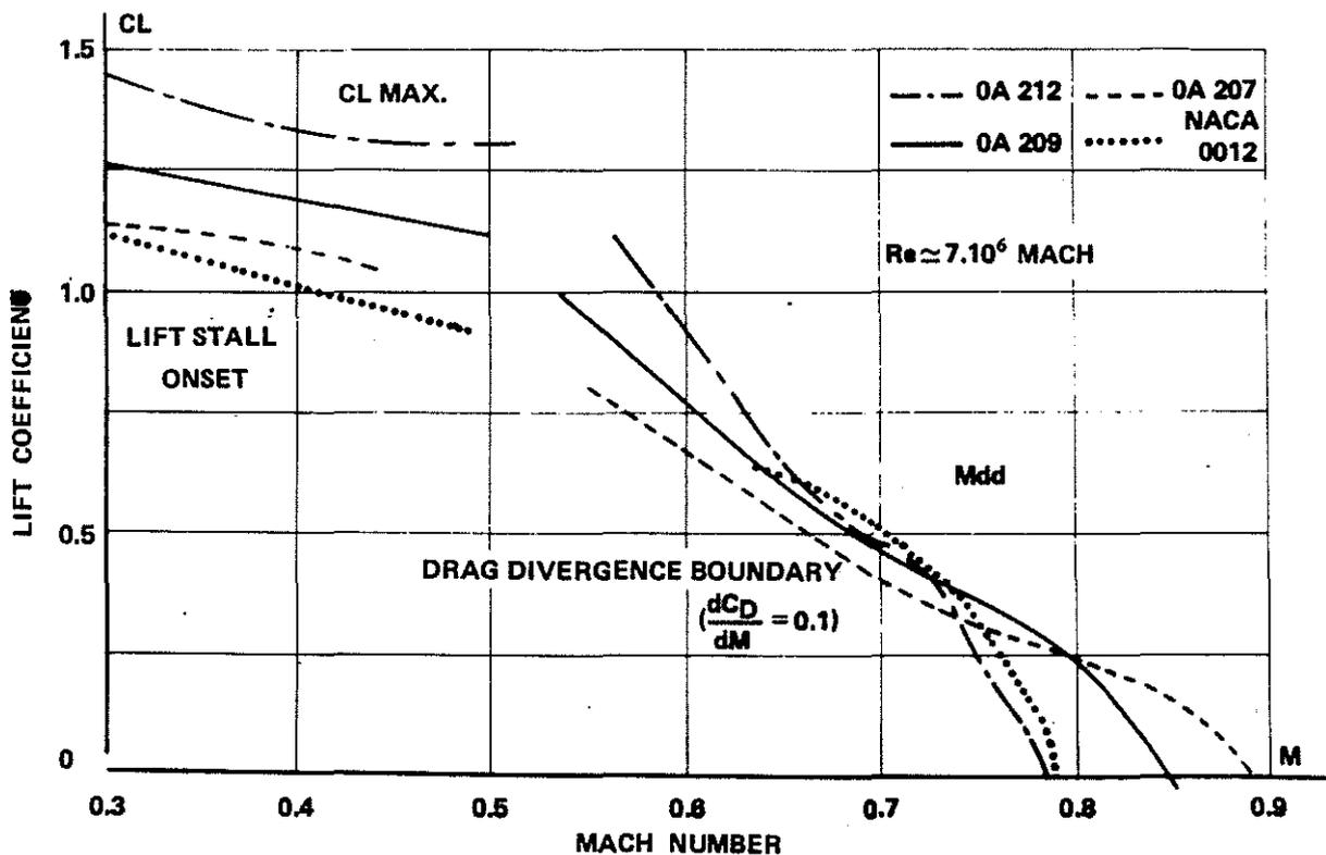
Figure 9 : OA2 AIRFOIL MAXIMUM LIFT AND DRAG DIVERGENCE MACH NUMBER COMPARED WITH NACA 0012
