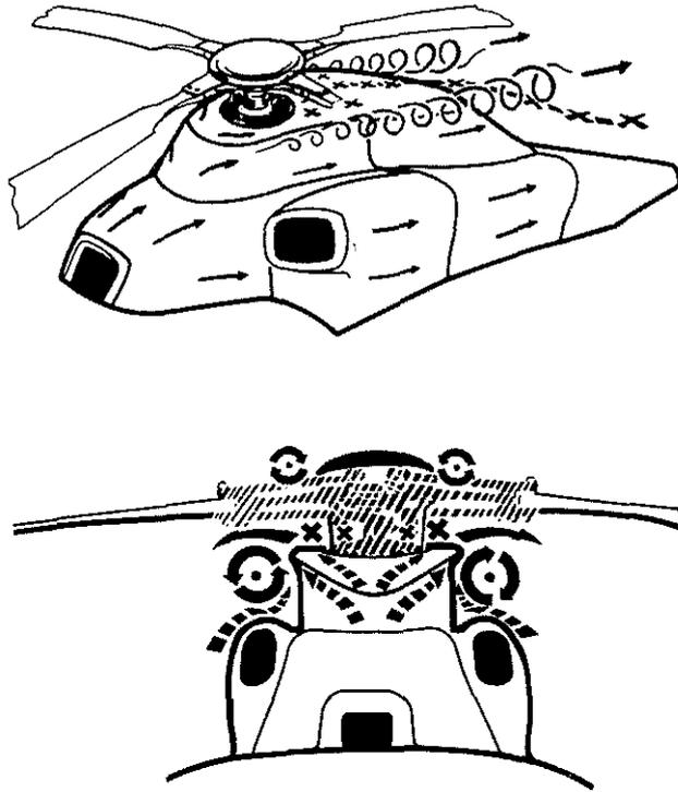
Figure 5 : PYLON FAIRING DESIGN (FLOW VISUALIZATION WIND TUNNEL TESTS)
