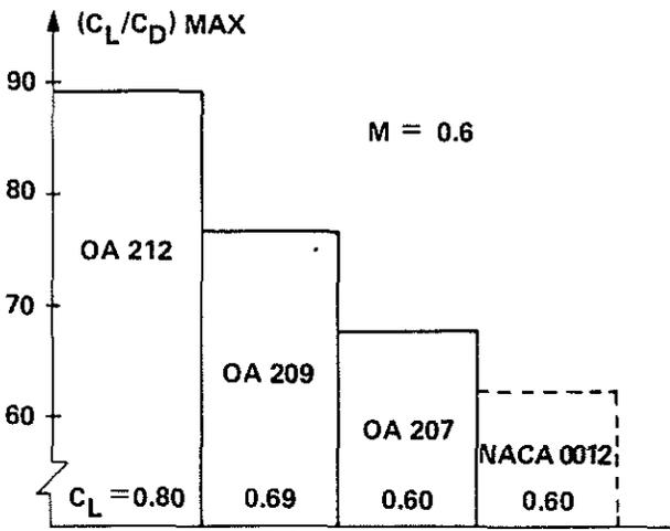
Figure 10: OA2 AIRFOIL LIFT TO DRAG RATIO COMPARED WITH NACA 0012
