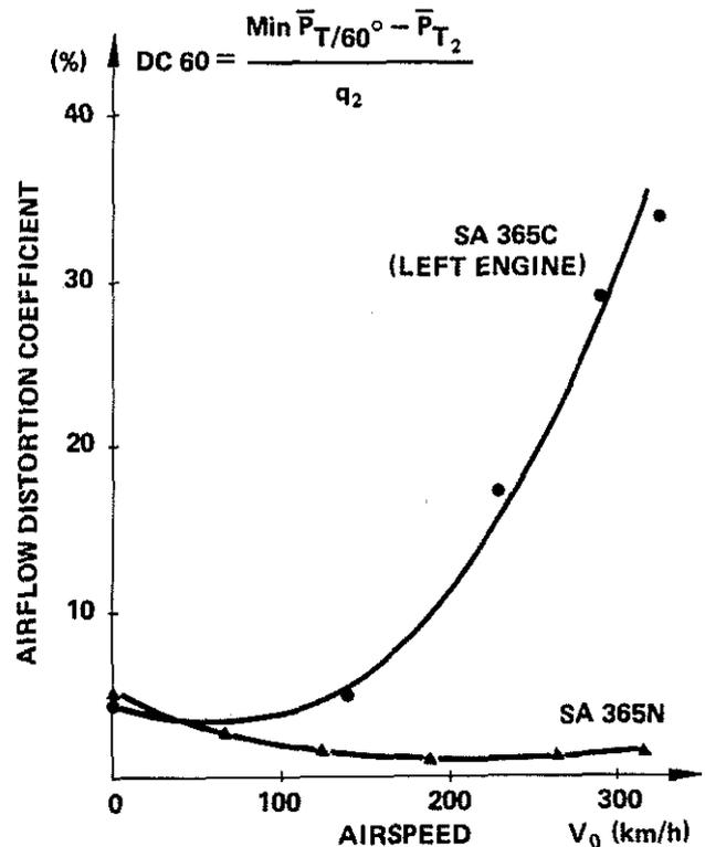
Figure 8 : AIR INTAKE DISTORSION VS. AIRSPEED (WIND TUNNEL TESTS)
