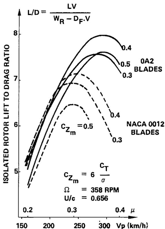
Figure 14 : OA2 ROTOR LIFT TO DRAG RATIO COMPARED WITH NACA 0012 BLADES
