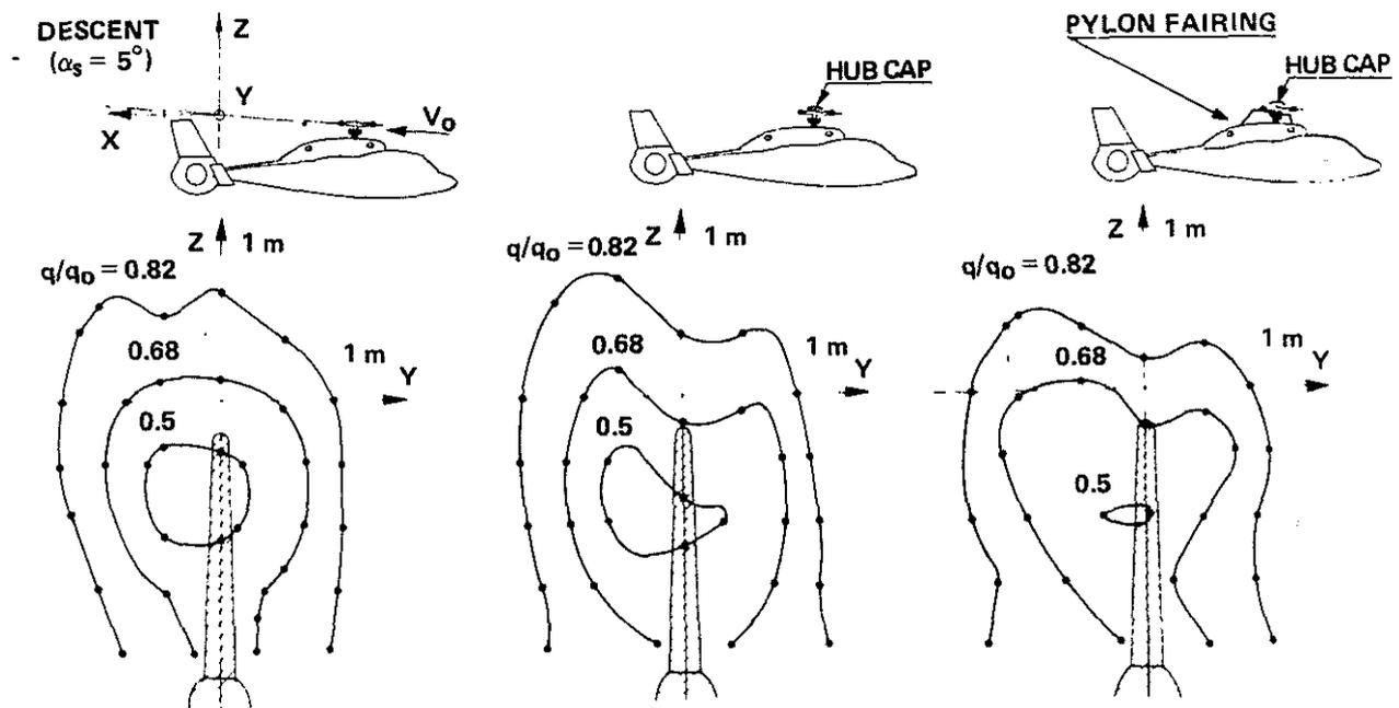
Figure 6 : MAIN ROTOR HEAD WAKE DYNAMIC PRESSURE MAP
