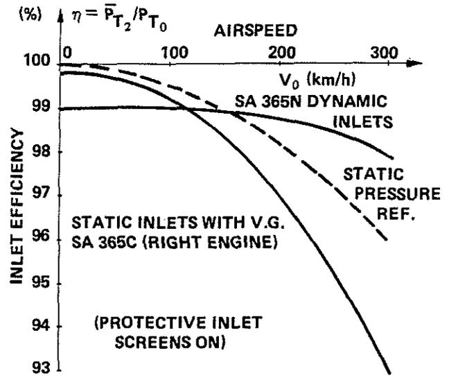
Figure 7 : ENGINE INLET EFFICIENCY VS. AIRSPEED (WIND TUNNEL TESTS)
