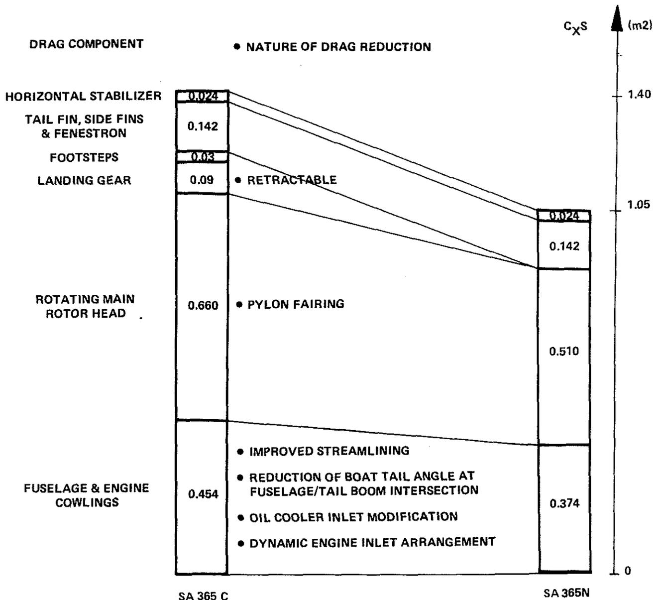
Figure 3: AIRFRAME PARASITE DRAG REDUCTION
