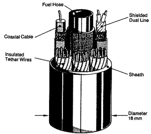
Fig. 7 Tethering Cable
