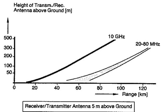
Fig. 9 Influence of Antenna Elevation on Range
