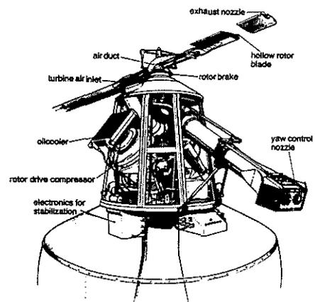
Fig. 5 Rotor Dynamic System
