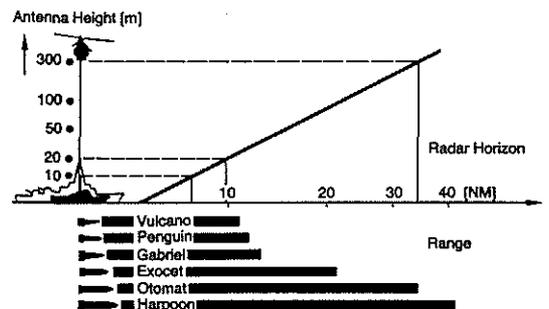
Fig. 12 Range of SS-Missiles and Target Acquisition Radar
