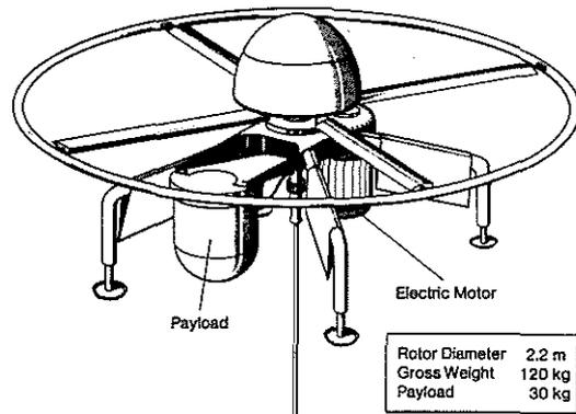
Fig. 16 Electric Rotorplatform
